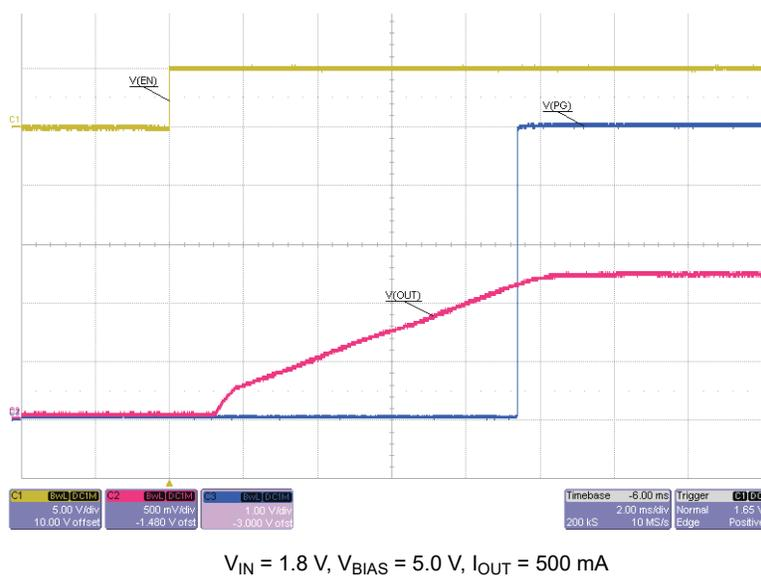
Figure 4-2. TPS74701 and TPS74801 Start-Up in 10 ms With PG
