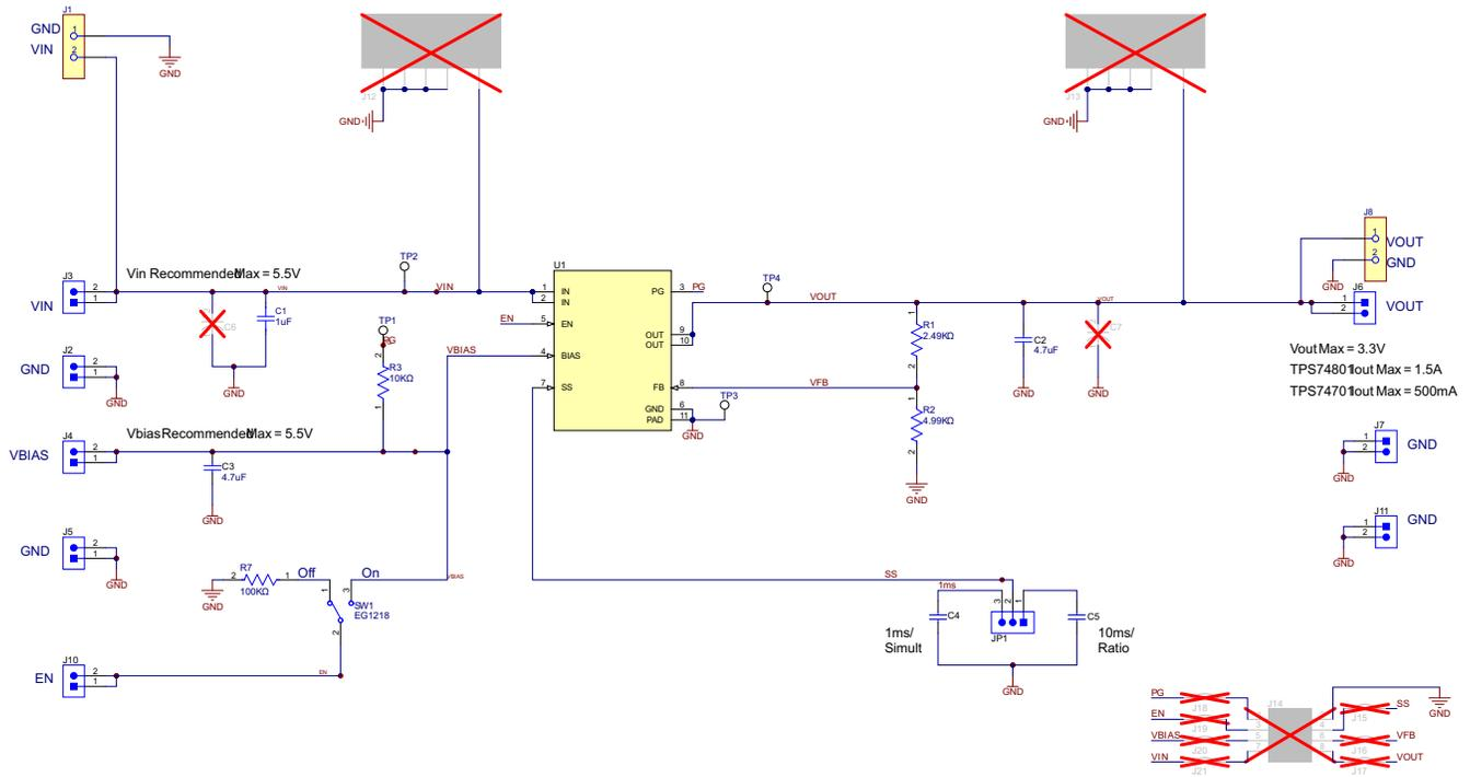
Figure 6-1. Schematic
