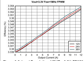
Figure 3-5. Load Regulation, VOUT = 3.3V, FPWM Mode
