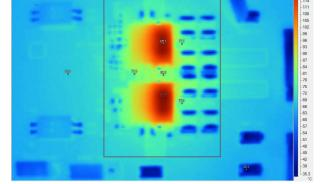
Figure 3-19. Infrared Thermal Image: VIN = 12V, IOUT = 12A
