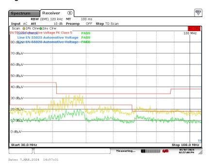
Figure 3-18. CISPR 25 Conducted Emissions: 30MHz to 108MHz
