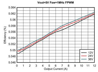
Figure 3-7. Load Regulation, VOUT = 5.0V, FPWM Mode
