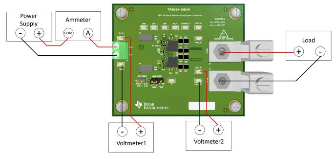
Figure 2-1. EVM Test Setup
