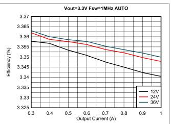
Figure 3-6. Load Regulation, VOUT = 3.3V, AUTO Mode
