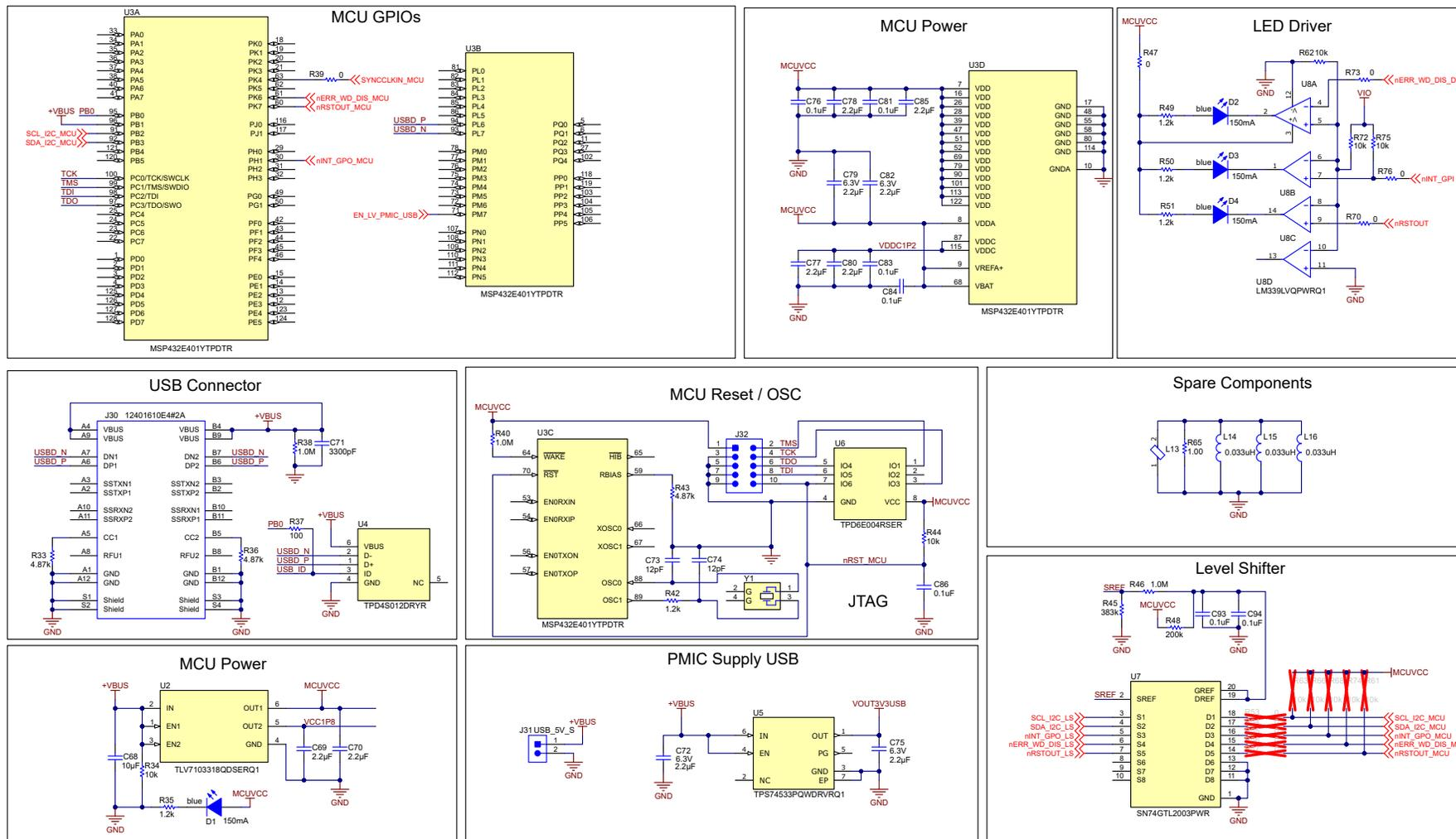
Figure 6-3. MCU Schematic
