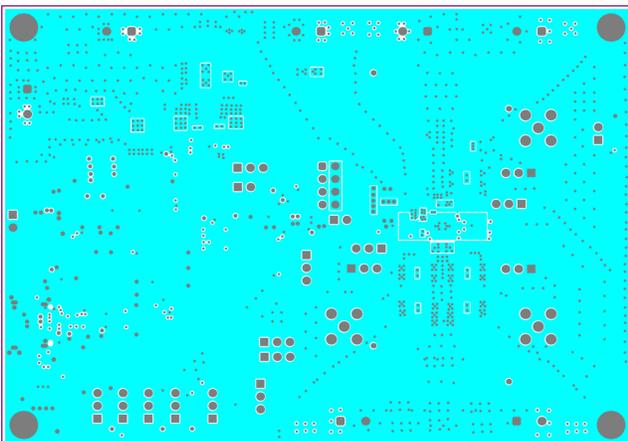
Figure 6-8. Layout of Ground Layer 2, Layer 5
