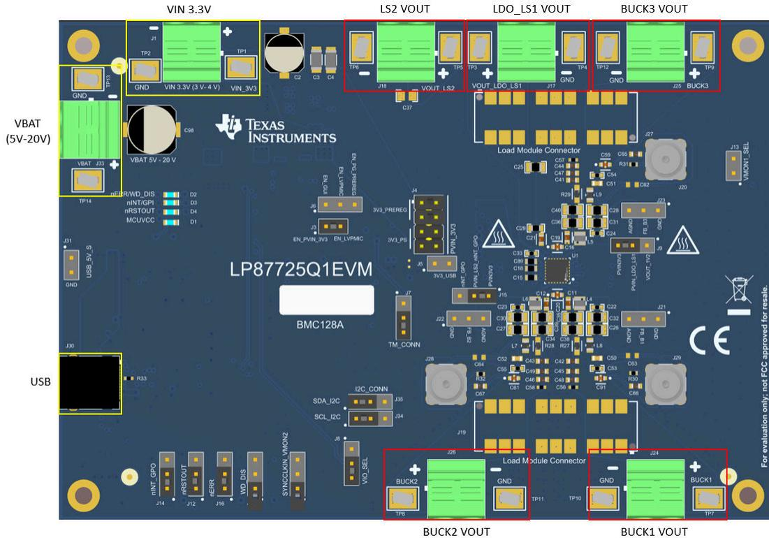
Figure 1-1. EVM Board Top View with Basic Connections and Default Jumpers
