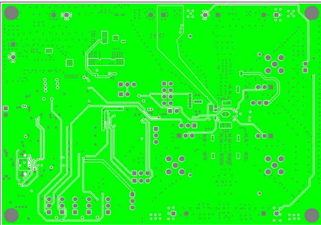
Figure 6-6. Layout of Signal Layer 1, Layer 3
