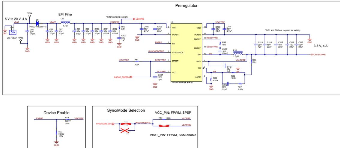
Figure 6-2. Preregulator Schematic
