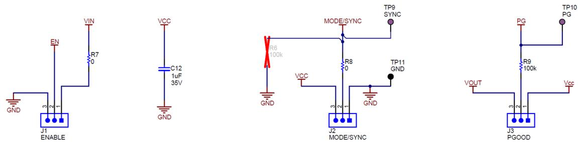
Figure 4-2. LMR66430-2EVM Schematic-Jumpers
