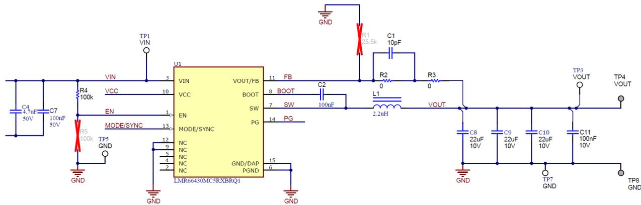
Figure 4-1. LMR66430-2EVM Schematic-Buck
