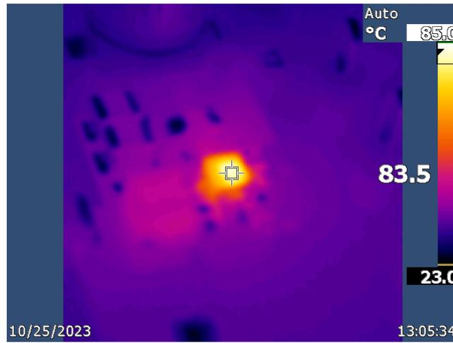
**Figure 3-3. Thermal capture with 3 A Load**
