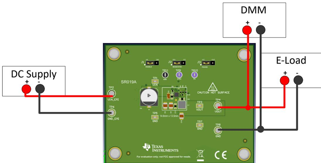
Figure 2-1. EVM Board Connections
