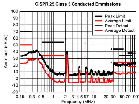
Figure 3-1. CISPR 25, Class 5, CE scan (150kHz to 108MHz)
