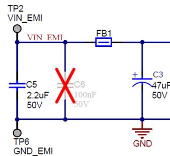
Figure 4-3. LMR66430-2EVM Schematic-Differential Filter
