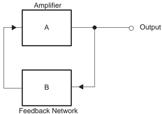
**Figure 4. Simple Form of an Oscillator Circuit**
