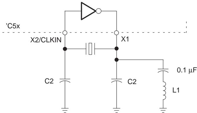
**Figure 16. Oscillator Circuit for Overtone Crystal Operation**
