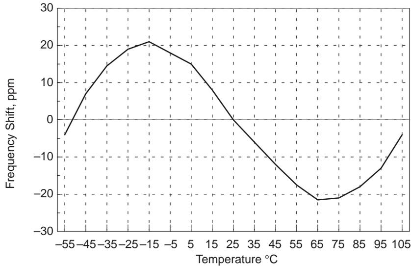
**Figure 19. Example Frequency-Temperature Characteristic of AT-Cut Crystals**
