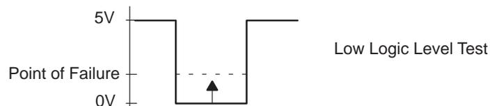
**Figure 11. Maximum Low Logic Level Voltage Input Signal**
