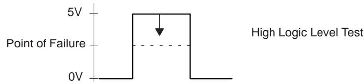
**Figure 10. Minimum High Logic Level Voltage Input Signal**
