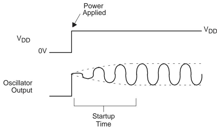
**Figure 18. Oscillator Startup**
