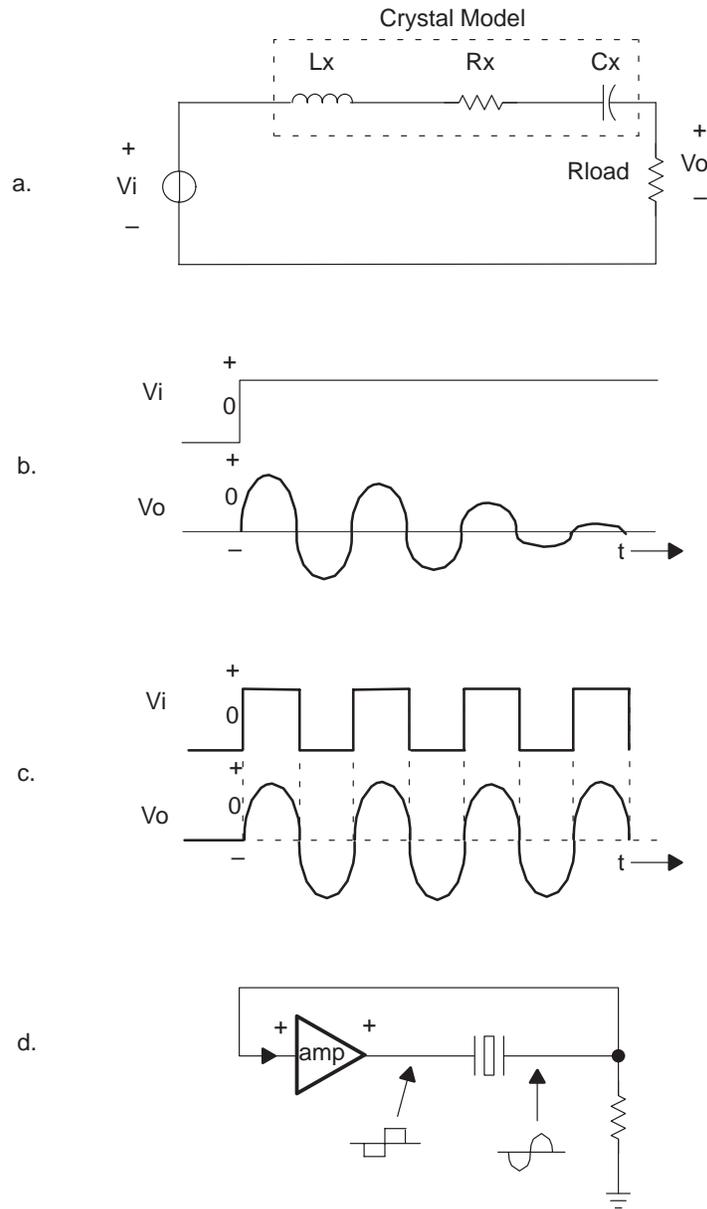
**Figure 3. Crystal Response to a Square-Wave Drive**
