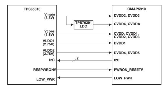
Figure 3. OMAP Low-Power System Architecture
