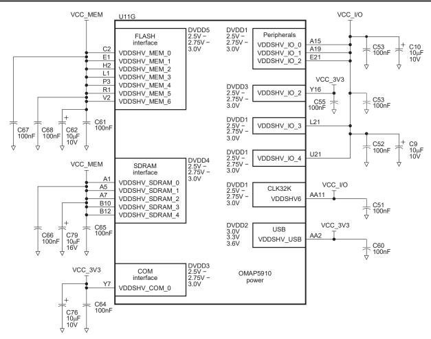
Figure 6. OMAP5910 I/O, Memory and USB Voltages
