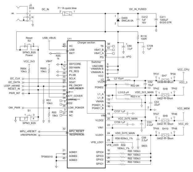
Figure 7. TPS65010 Power Management Circuit
