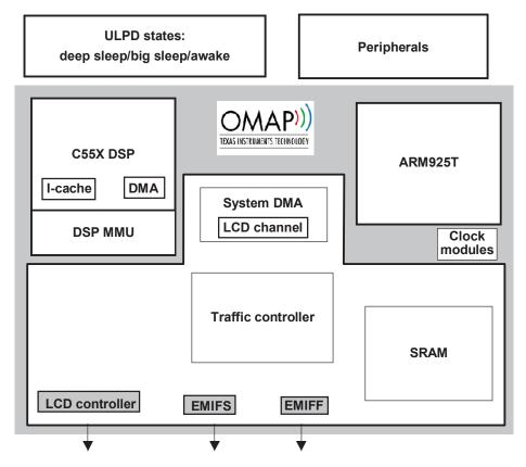
Figure 1. OMAP5910 Device Architecture
