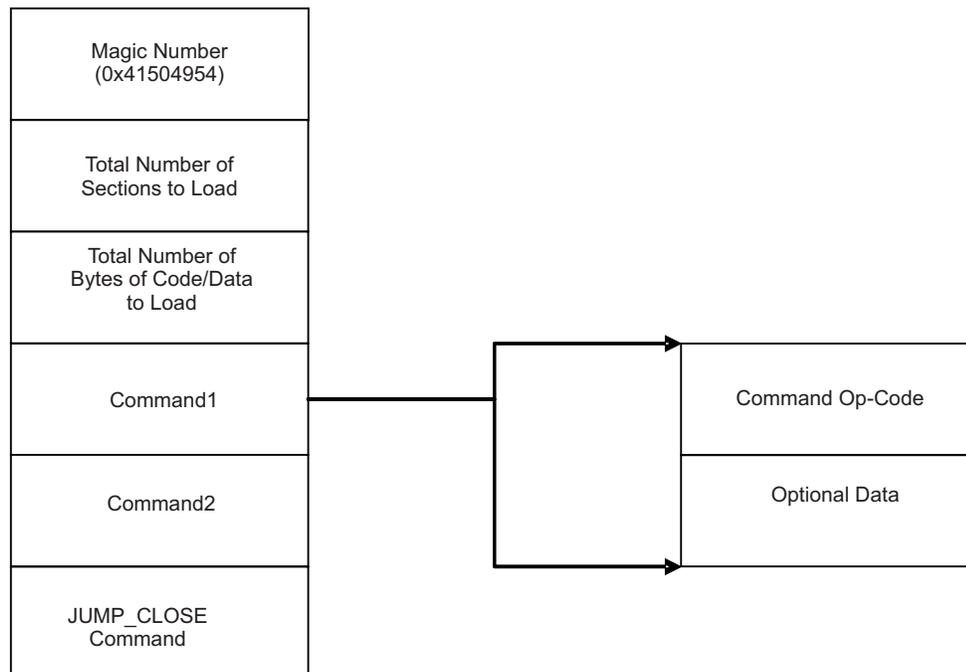
**Figure 3. Basic Structure of Application Image Script**
