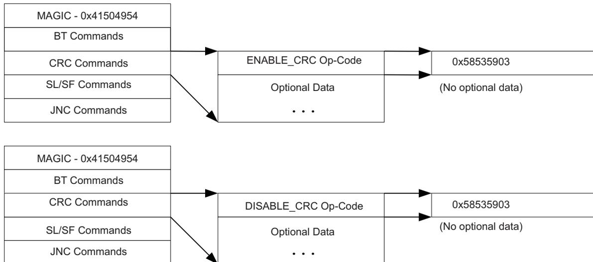
Figure 11. Structure of Enable CRC/Disable CRC Commands
