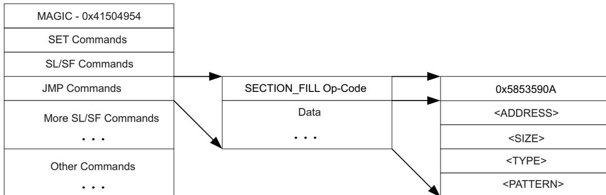
Figure 8. Structure of Section Fill Command
