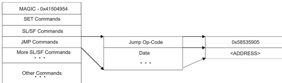
Figure 9. Structure of Jump Command
