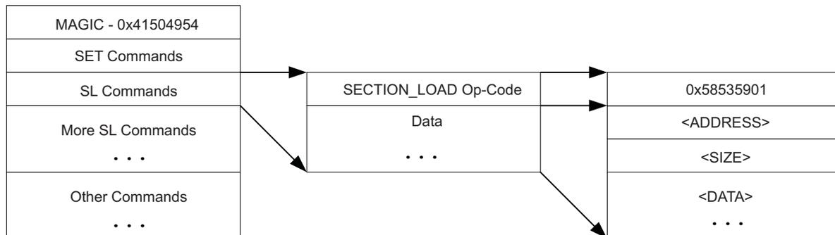
**Figure 7. Structure of Section Load Command**
