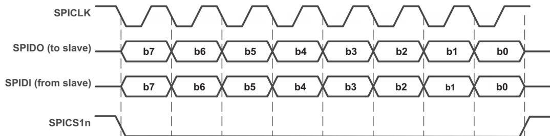
**Figure 1. SPI Transfer With Polarity = 1, Phase = 0**
