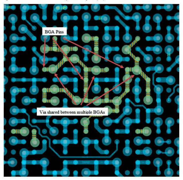
Figure 5-1. Via Sharing for VDD\_CORE Domain
