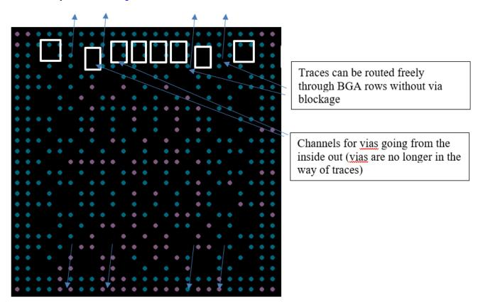
Figure 2-1. AM62xSiP BGA array with Via Channels
