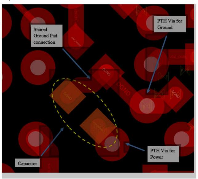
Figure 10-1. AM62XSiP SK EVM Output Capacitor Placement for CAP VDDS0
