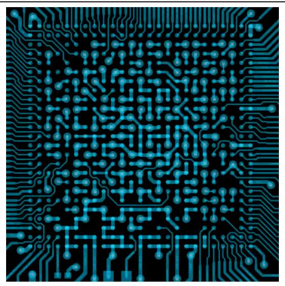
Figure 12-1. AM62xSiP with Complete Signal and Power Escapes
