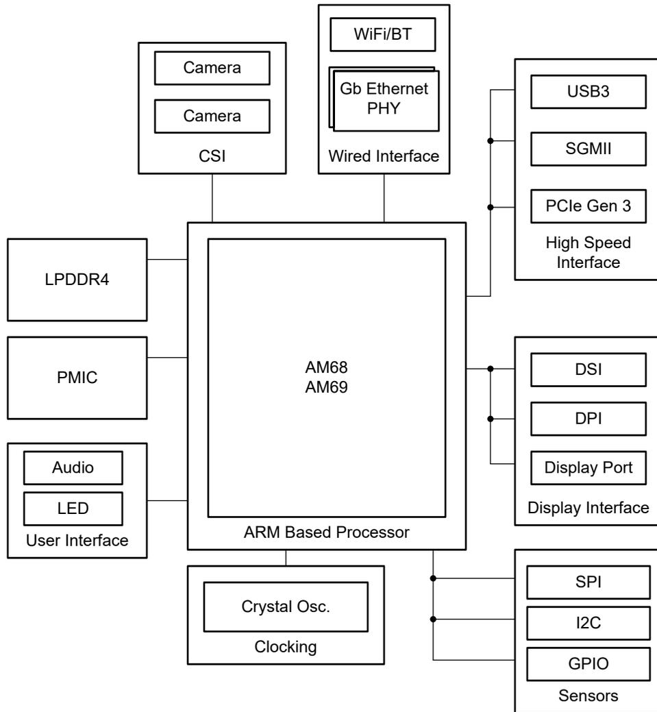
**Figure 4-3. Single Board Computer Block Diagram**
