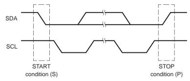
The I2C-bus is considered busy after a START condition and before a subsequent STOP condition. The bus busy (BB) bit of ICSTR is 1. The bus is considered free between a STOP condition and the next START condition. The BB is 0.
