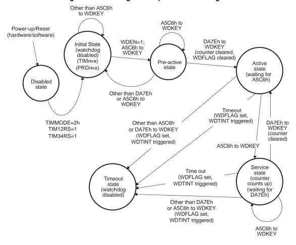
Figure 10. Watchdog Timer Operation State Diagram
