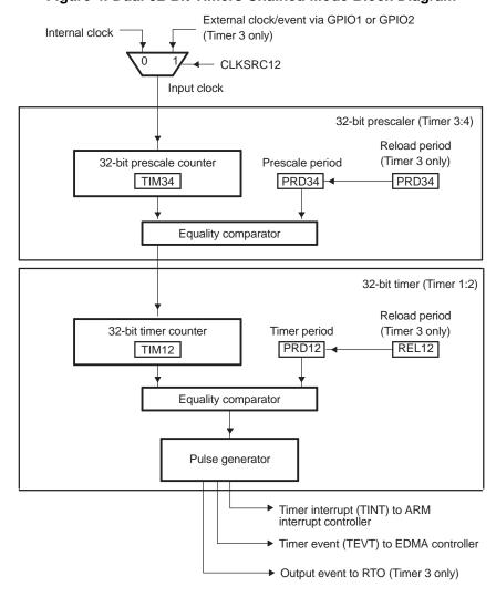
Figure 4. Dual 32-Bit Timers Chained Mode Block Diagram
