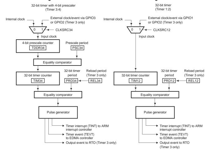
Figure 6. Dual 32-Bit Timers Unchained Mode Block Diagram
