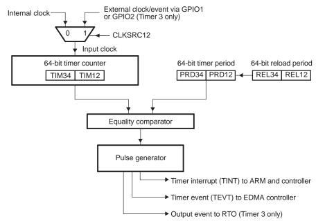
Figure 3. 64-Bit Timer Mode Block Diagram
