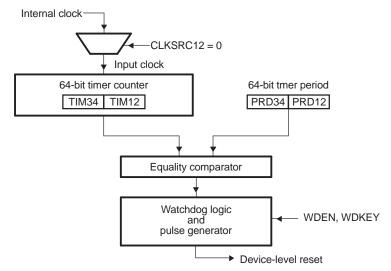
Figure 9. Watchdog Timer Mode Block Diagram
