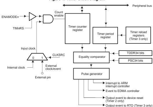
Figure 1. Timer Block Diagram
