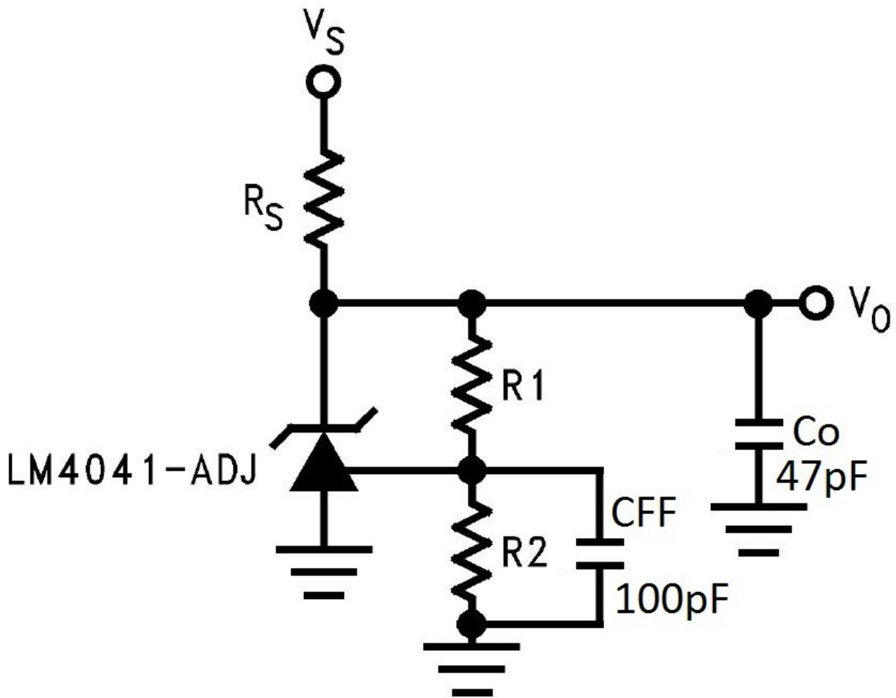
**Figure 9. Final Schematic of LM4041-N as a 2.5V Voltage Reference**
