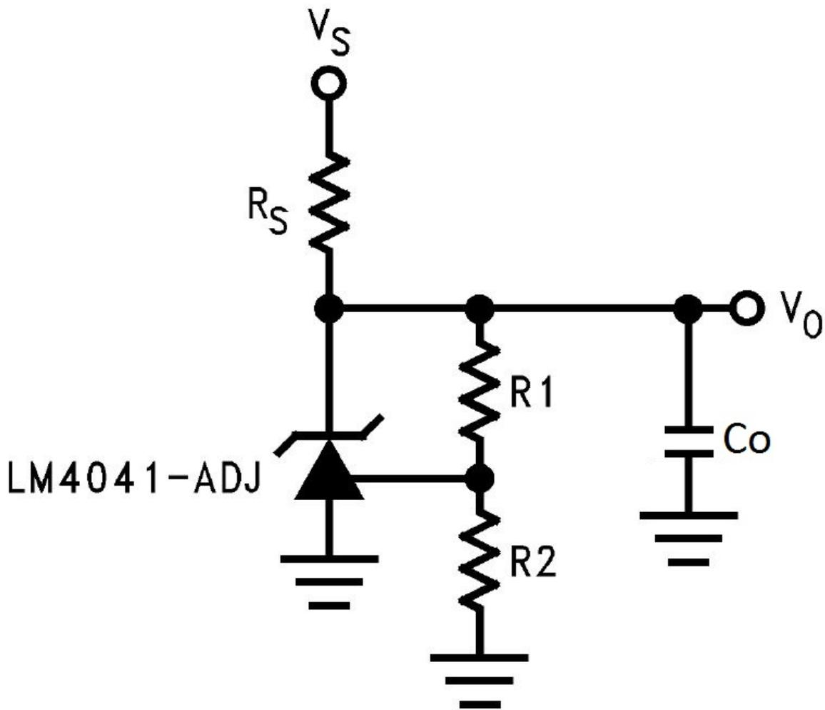
**Figure 3. LM4041-N Typical Application Circuit**
