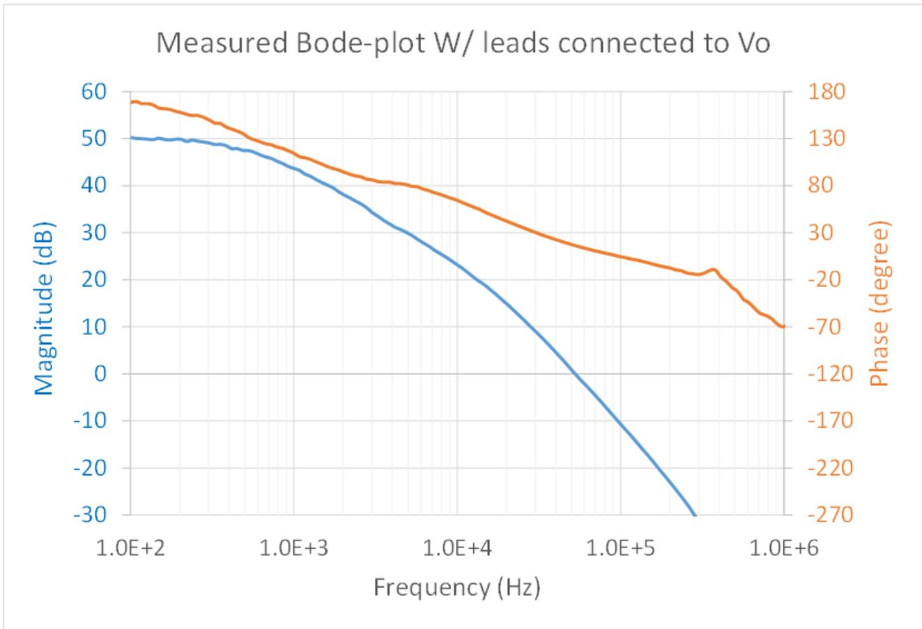
**Figure 8. Measured Bode Plot with Reference Leads Connected to  $v_o$**
