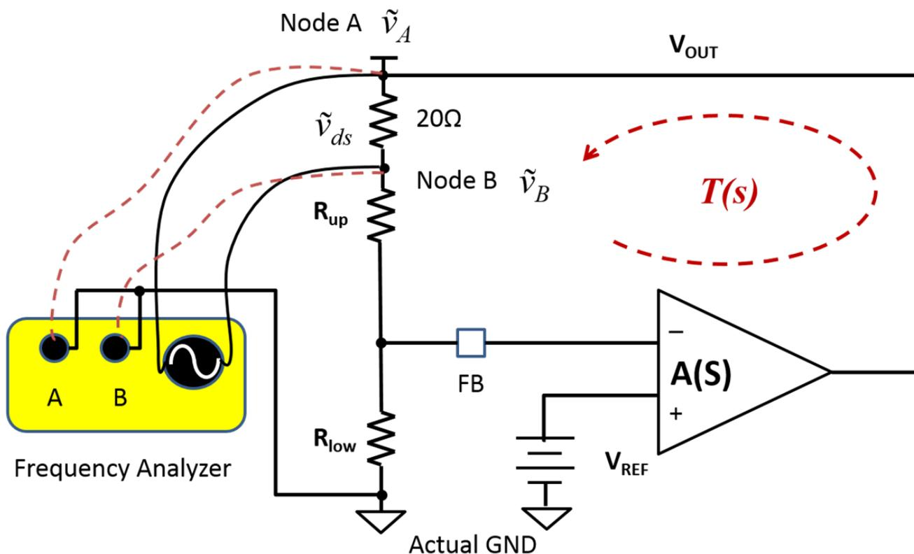
Figure 1. Typical T Measurement Setup
