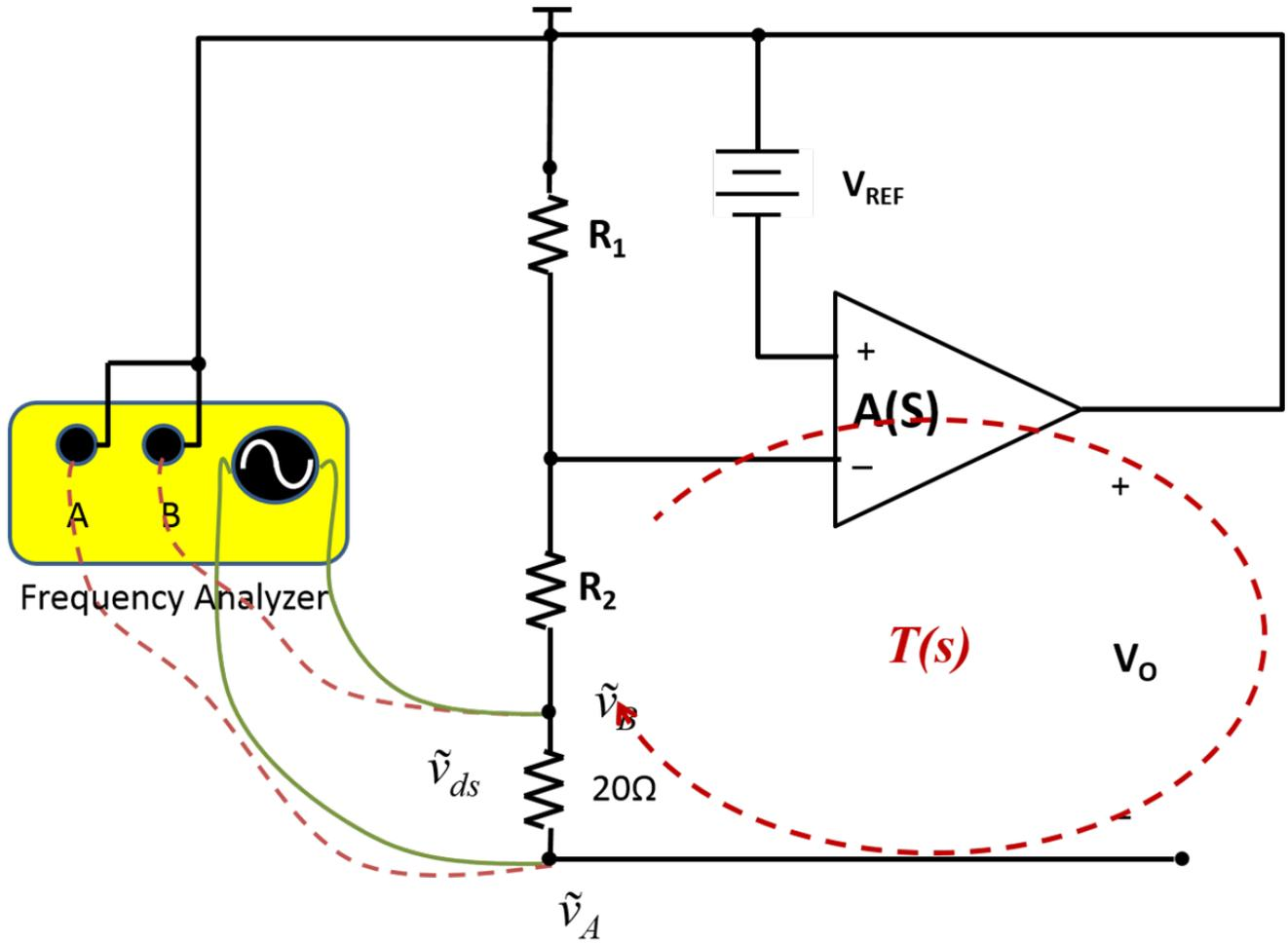
**Figure 7. Small-signal Model Referring to the Output**
