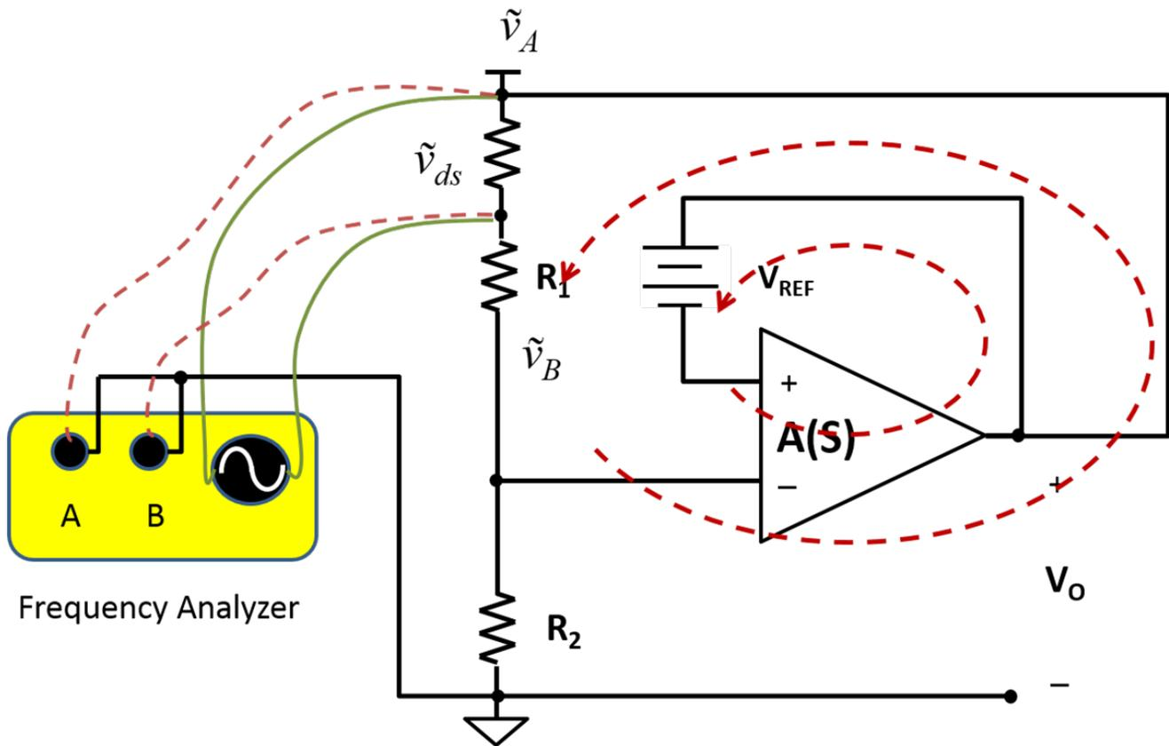
**Figure 6. Small-signal Model Referring to Ground**
