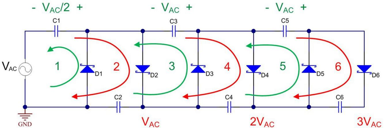
**Figure 1. A Voltage Multiplier Uses an Alternating Current (AC) Voltage with Diodes and Capacitors in a Cascade**
