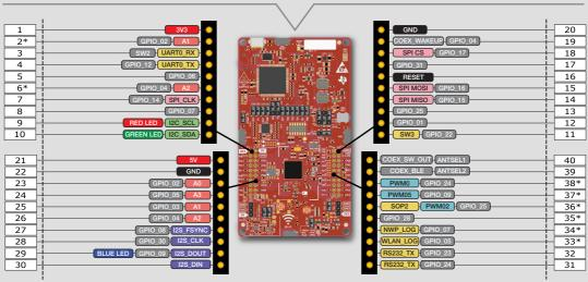
\*These pins are not connected to the Launchpad Connector by default.
