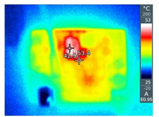
Figure 2-8.  $20V_{IN}$  to 30V Battery Short Circuit Thermal Test
