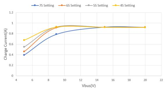
Figure 2-3. Charge Current Across  $V_{\mbox{\scriptsize IN}}$  and Battery Voltage
