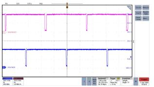
Figure 3-10. Buck-Boost Mode Switching Node Waveform V<sub>IN</sub> = 20V, Battery Voltage = 20V
