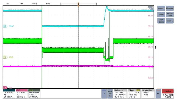
Figure 3-11. Short-Circuit Protection and Recovery at 20V<sub>IN</sub> and 30V Battery Condition
