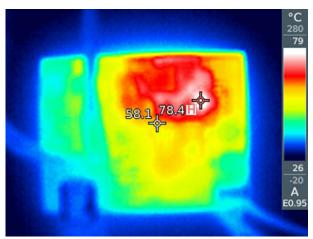
Figure 2-6. 15V<sub>IN</sub> to 30V Battery Charge Thermal
