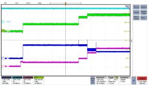
Figure 3-2. Input Source Voltage Transition up From 5V to 9V, 15V, 20V USB PD Source Charge 7S Battery 30V, 900mA
