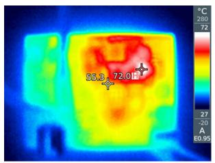
Figure 2-7. 20V<sub>IN</sub> to 30V Battery Charge Thermal
