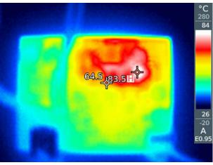
Figure 2-5.  $9V_{\text{IN}}$  to 30V Battery Charge Thermal
