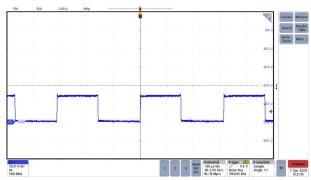
Figure 3-7. Boost Mode Switching Node Waveform Figure 3-8. Boost Mode Switching Node Waveform V<sub>IN</sub> = 15V, Battery Voltage = 30V
