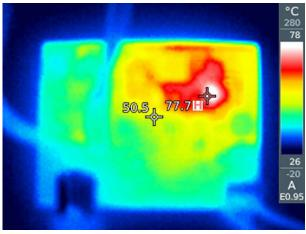
Figure 2-4. 5V<sub>IN</sub> to 30V Battery Charge Thermal
