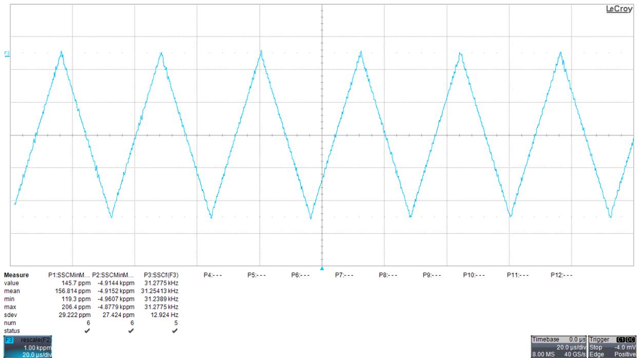
Figure 2. Spread Spectrum Clocking of TUSB9261-Q1. The SSC deviation was -4.9607kPPM and the modulation rate was 31.254kHz.
