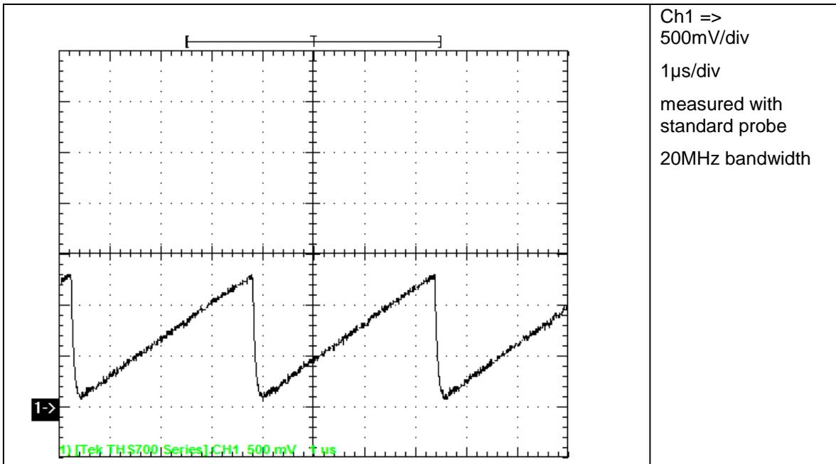
**Figure 32, ramp at RC oscillator**
