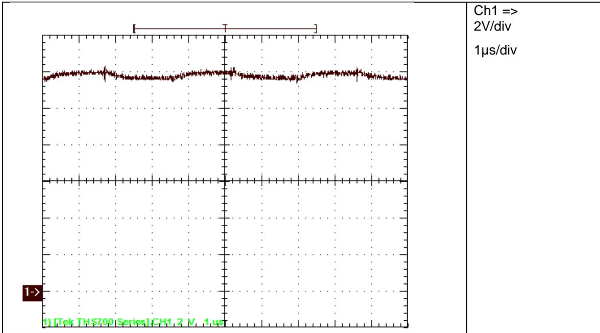
**Figure 31, voltage stress at clamping capacitors is equal to input voltage**
