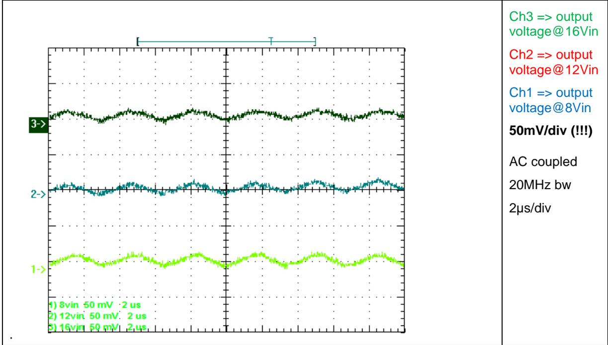
Figure 17, continuous output current results in lowest ripple
