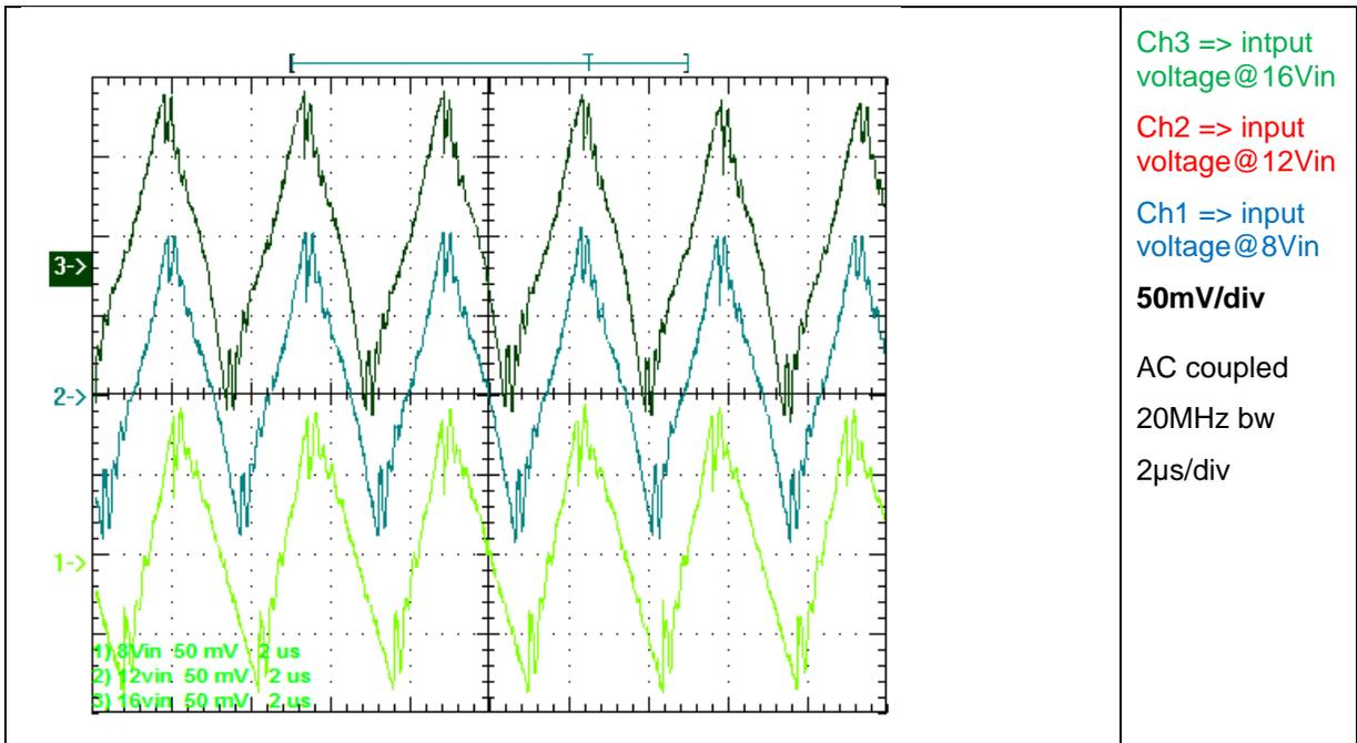
Figure 18, pulse current across input capacitors, watch reflected ripple
