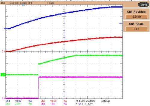
Ch1: 18V, Ch2:12V, Ch3: 3.3V, Ch4: 1.8V (4msec/div, 20MHz) → all outputs unloaded
