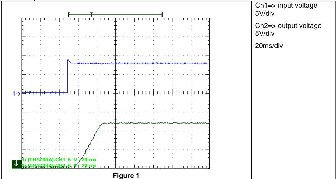
The startup waveform is shown in the Figure 2. The input voltage was set at 12V, with 1A load at the output.
