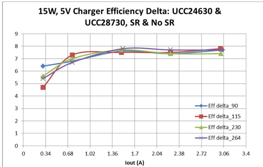
Figure 8. Efficiency improvement with SR over line and 10% to 100% load.
