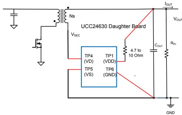
Figure 2. Demonstration card connection to existing circuit shown
