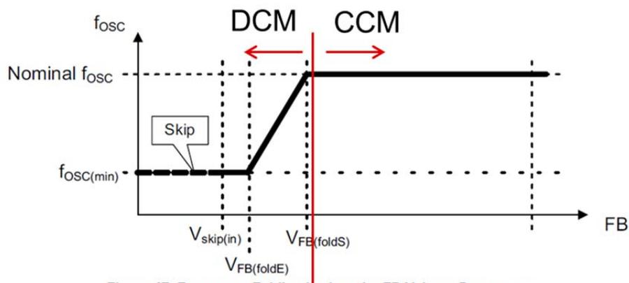
Figure 47. Frequency Foldback when the FB Voltage Decreases
