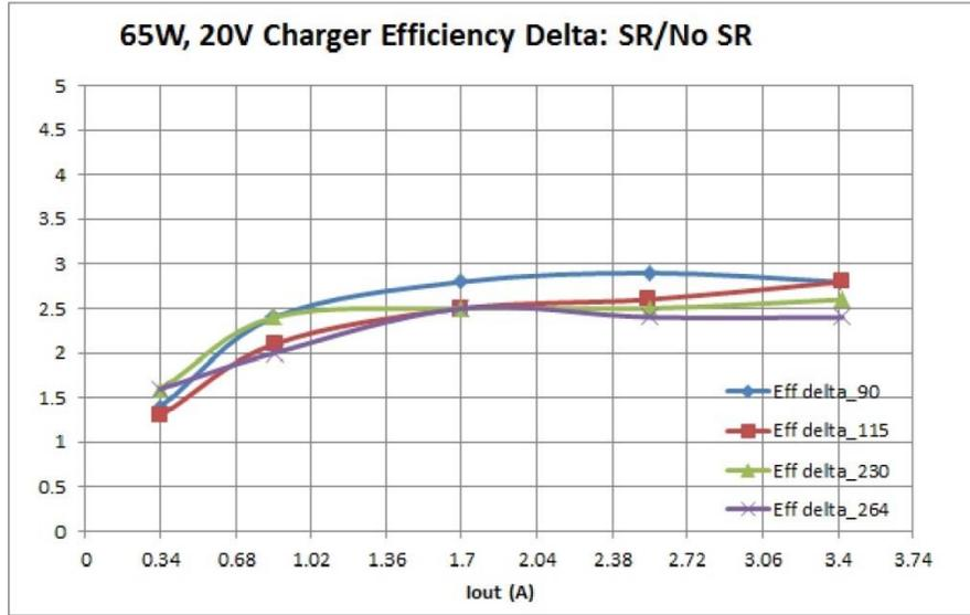
Figure 7. Efficiency improvement with SR over line and 10% to 100% load.
