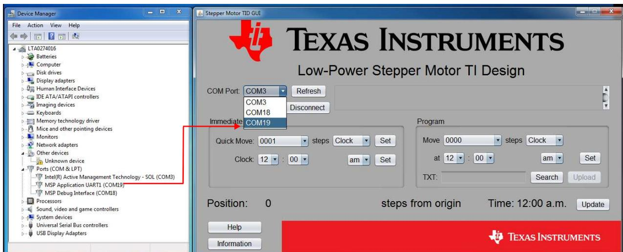
**Figure 11. GUI COM Port Settings**
