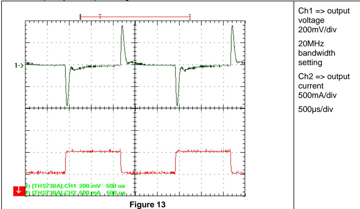
If transient response <3% is needed increase output capacitance
