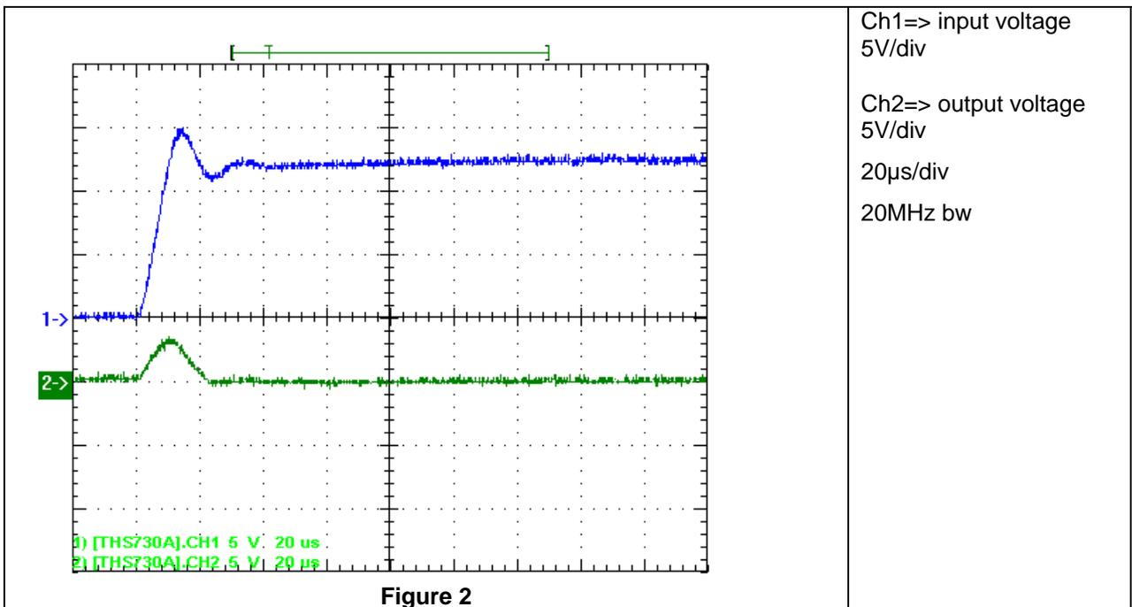
The startup waveform is shown in the Figure 3. The input voltage was set at 12V, with 0A load at the output.
