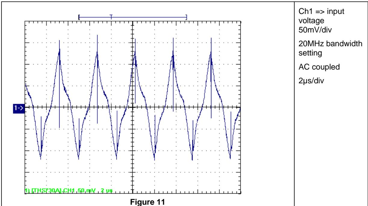
The input ripple voltage is shown in **Error! Reference source not found.** The image was taken with 0.5A load 12V at the input. The waveforms were captured timely separate.
