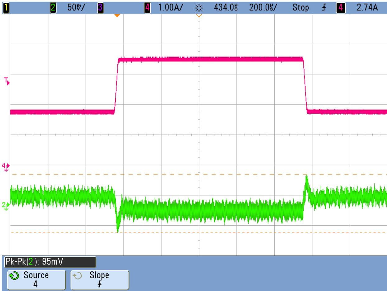
$V_{IN}=4.5V$ , 3V3 Channel: 1.75A-3A-1.75A
