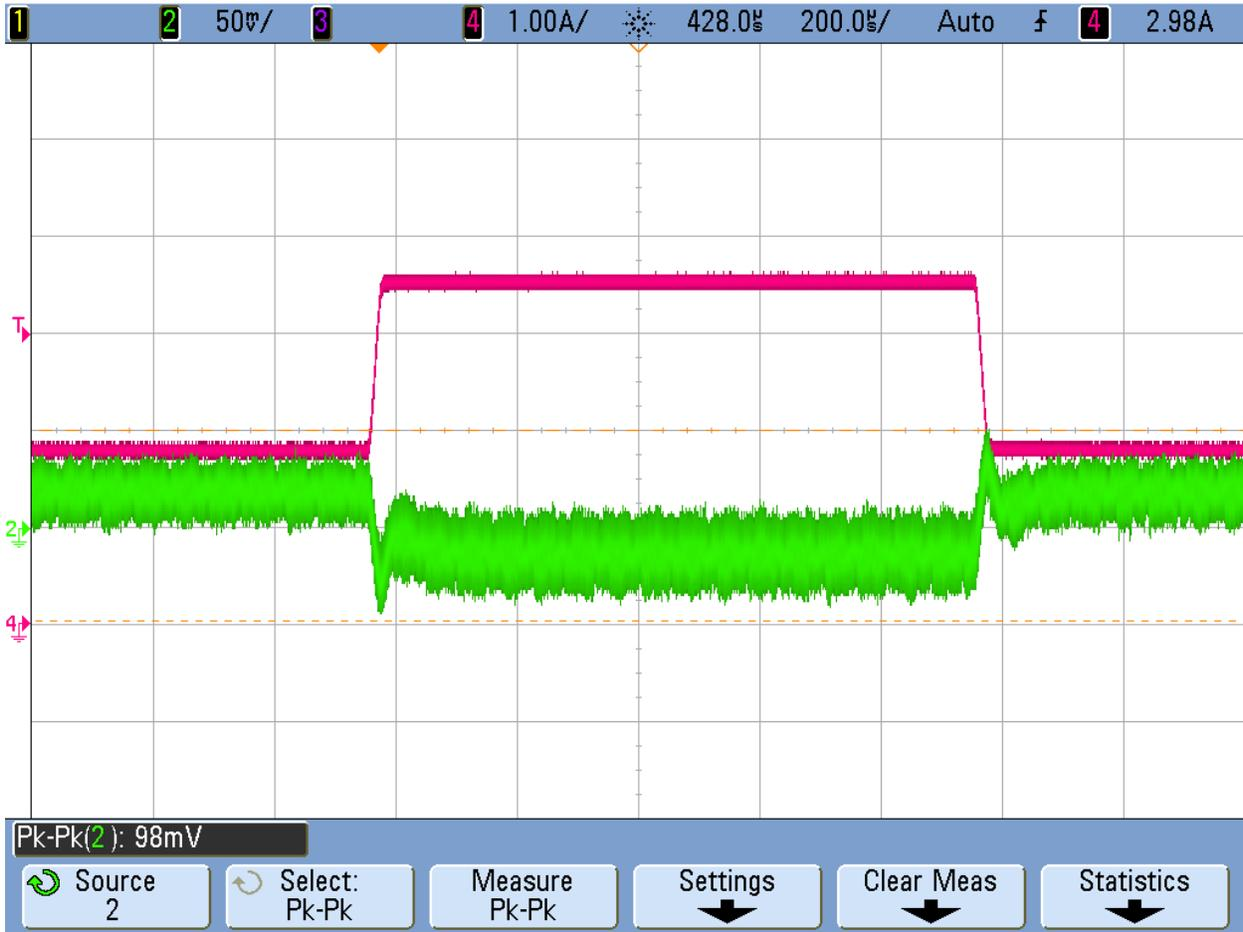
$V_{IN}=18V, 3V3$  Channel: 1.75A-3A-1.75A
