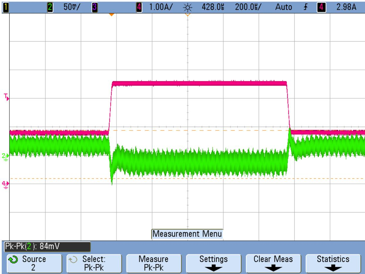
$V_{IN}=9V$ , 3V3 Channel: 1.75A-3A-1.75A
