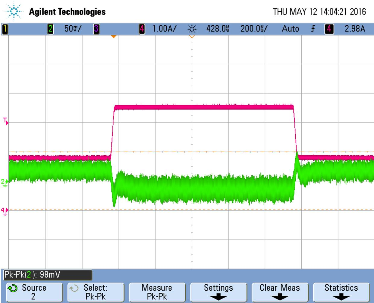
$V_{IN}=12V$ , 3V3 Channel: 1.75A-3A-1.75A
