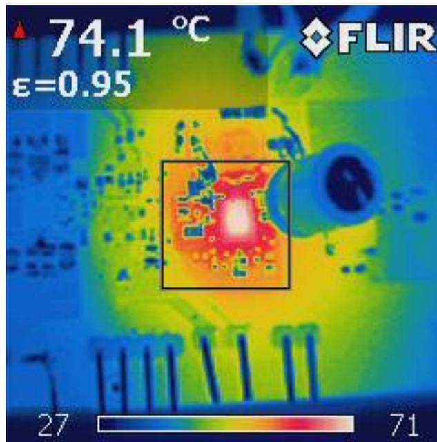
IR thermal image taken at steady state at Full load and  $V_{IN} = 12V$  with no airflow
