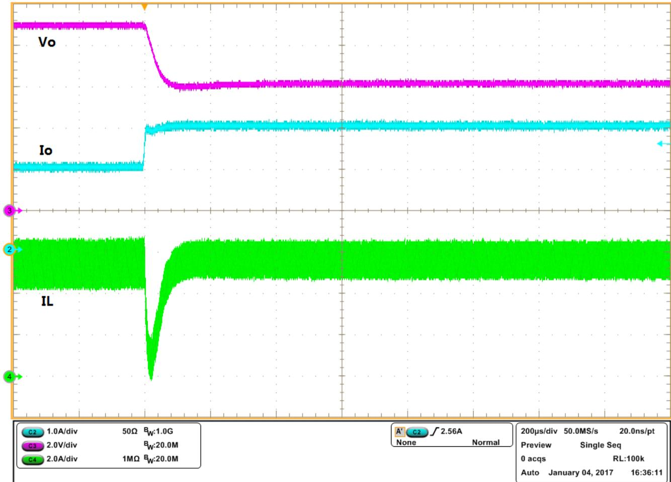
Figure 5. Output Current Limit Waveforms at  $V_o = 9\text{ V}$  ( $I_o = 2\text{ A}$  to  $3\text{ A}$ )
