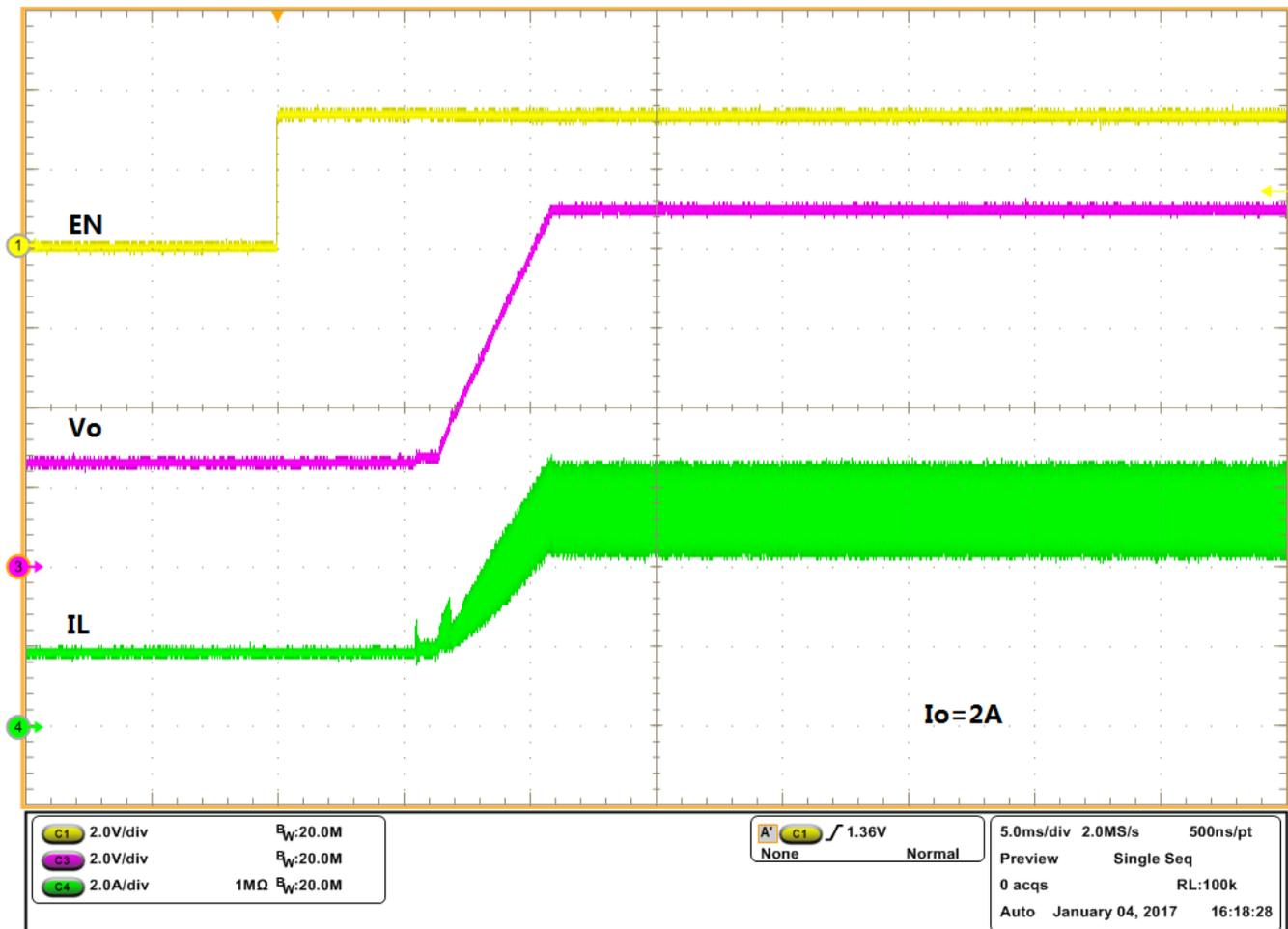
Figure 3. Start-up Waveforms at  $I_o = 2\text{ A}$  ( $V_o = 9\text{ V}$ )
