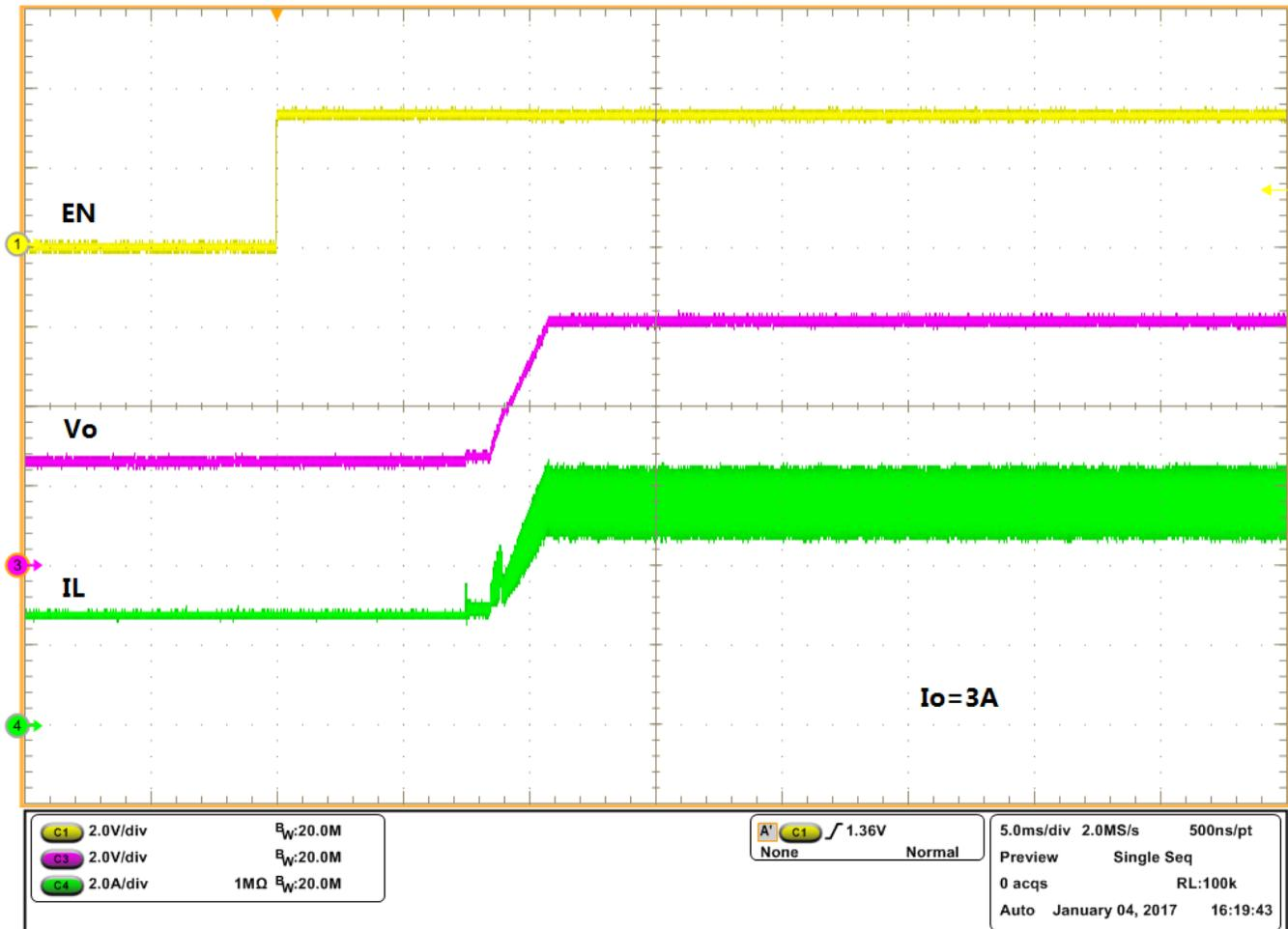
Figure 4. Start-up Waveforms at  $I_o = 3\text{ A}$  ( $V_o = 9\text{ V}$ )
