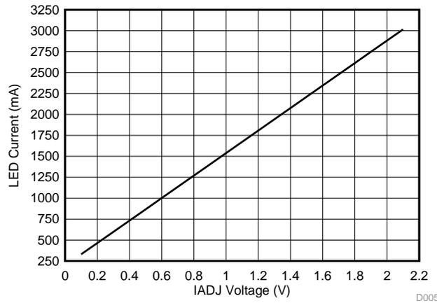
Figure 14. LED Current versus IADJ Voltage (IADJ Varied From 0.1 V to 2.1 V)
