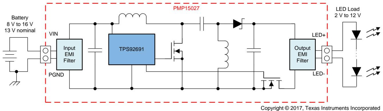
**Figure 1. PMP15027 Block Diagram**
