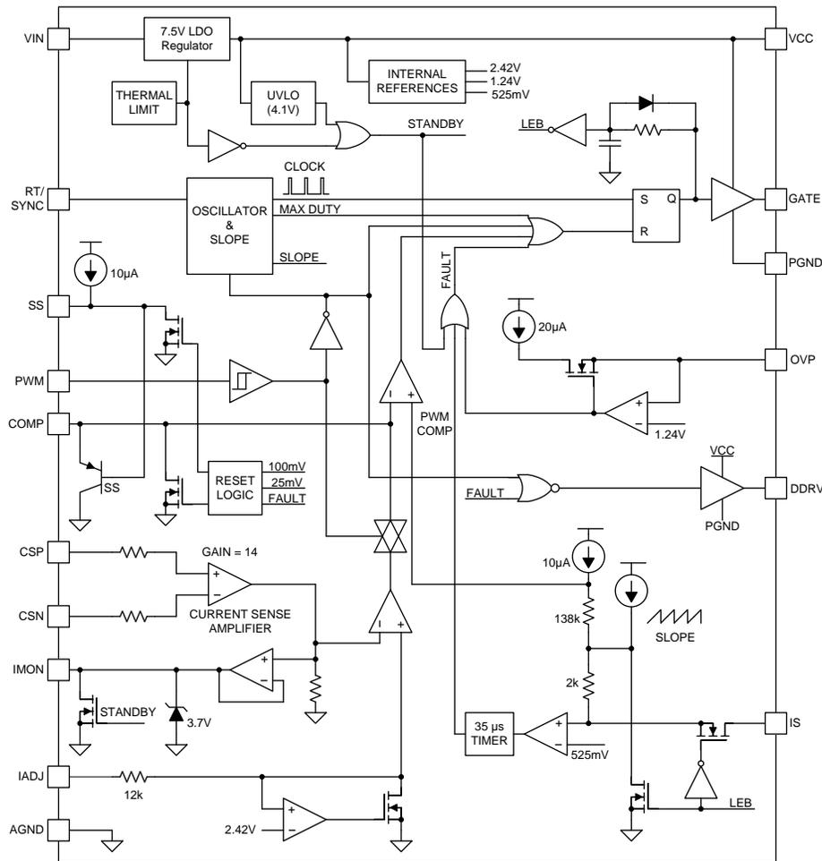
**Figure 2. TPS92691 Block Diagram**
