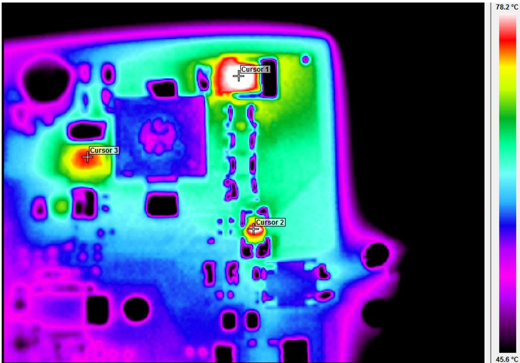
Figure 16. Thermal Scan—Top-View (Power Components):  $V_{\text{IN}} = 13 \text{ V}$ , Six LEDs,  $I_{\text{LED}} = 3 \text{ A}$
