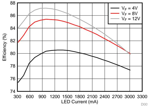
Figure 10. 9-V Input Efficiency versus LED Current
