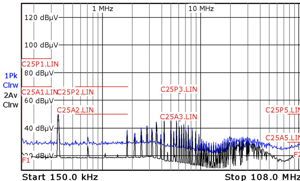
Figure 4. CISPR-25 Class 3 Conducted EMI Scan (C25Px: Peak Limits, C25Ax: Average Limits)
