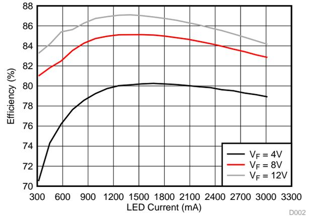
Figure 11. 13-V Input Efficiency versus LED Current
