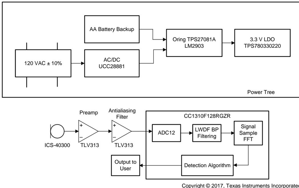
**Figure 1. TIDA-01519 Block Diagram**
