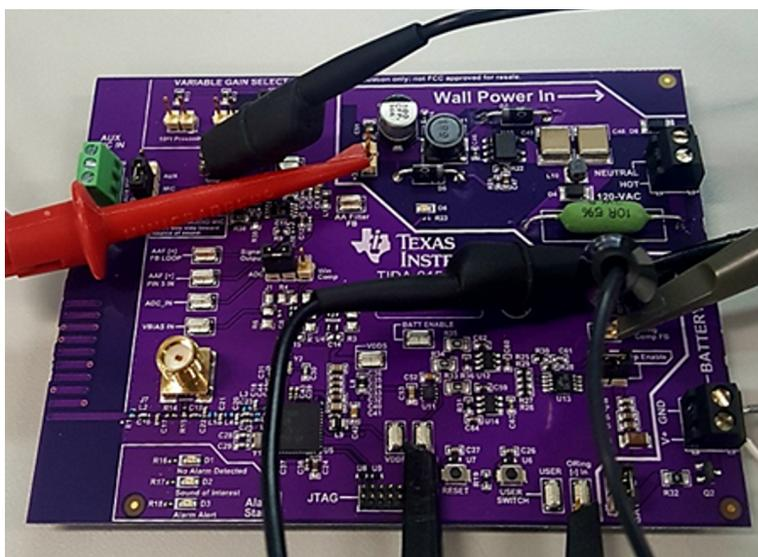
Figure 47. Test Setup of Power Source ORing
