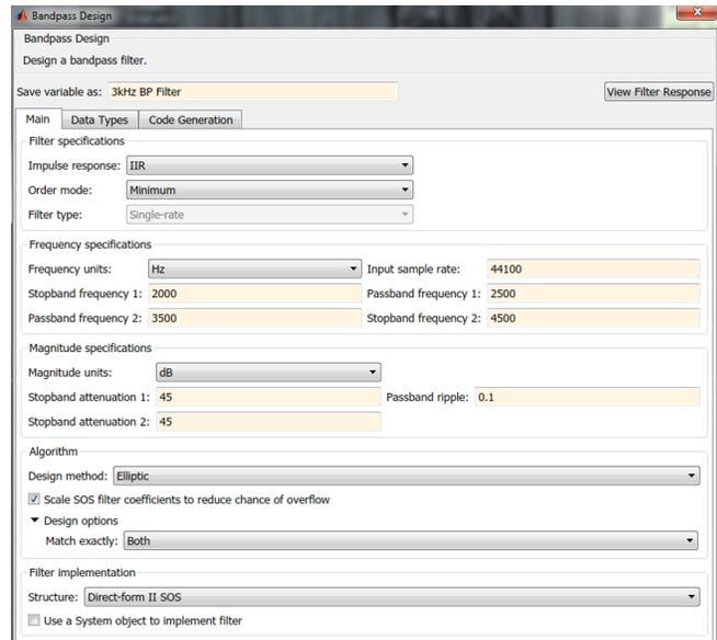
Figure 33. Main Graphical Interface of MATLAB Filter Design
