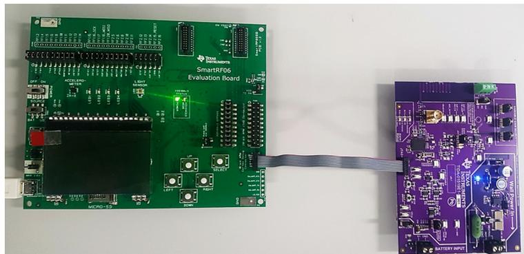
**Figure 44. Proper SmartRF06 to TIDA-01519 Board Connection**
