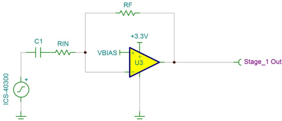
Figure 20. TIDA-01519 Circuit Structure of Audio Amplification
