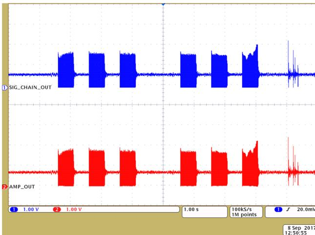
Figure 50. Signal Chain Response at 5-ft Proximity
