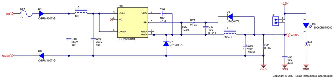
Figure 9. TIDA-01519 120-V AC to DC Schematic
