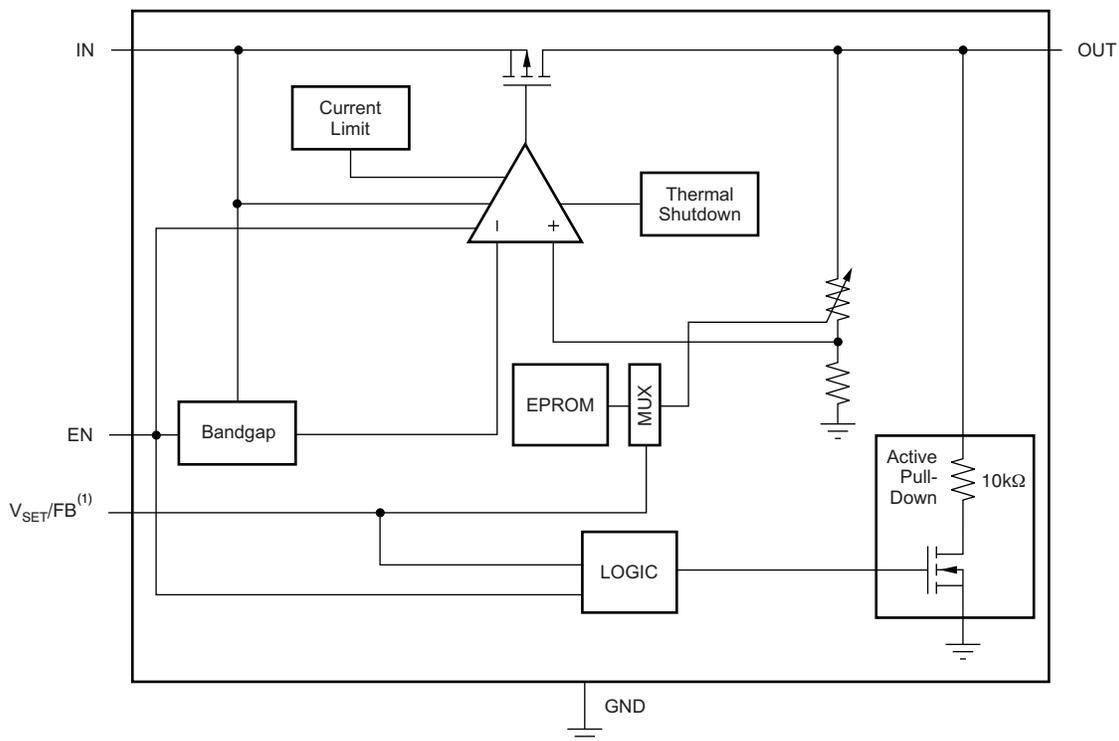
**Figure 5. TPS780330220DRVR Functional Block Diagram**
