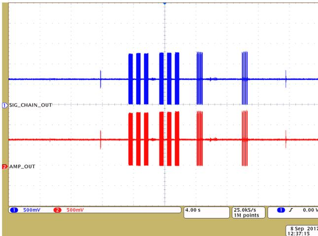
Figure 48. Signal Chain Response at 1-ft Proximity
