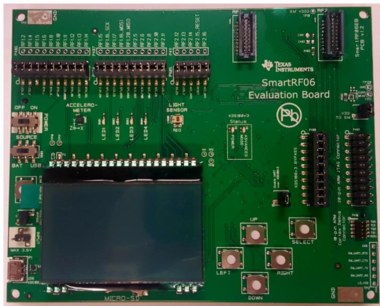
Figure 43. SmartRF06 Evaluation Board
