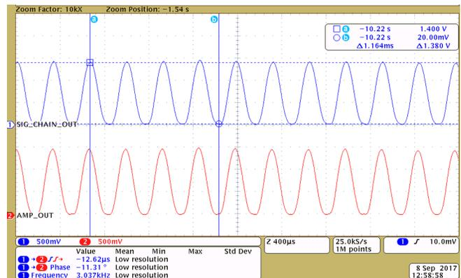
Figure 51. Delay, Phase, and Frequency Data Acquisition at 5-ft Proximity
