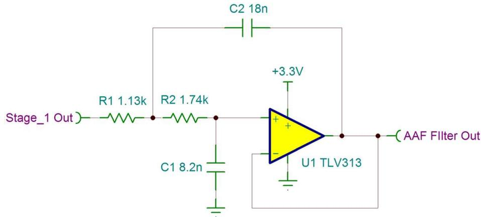
Figure 24. TIDA-01519 Antialiasing Filter Circuit
