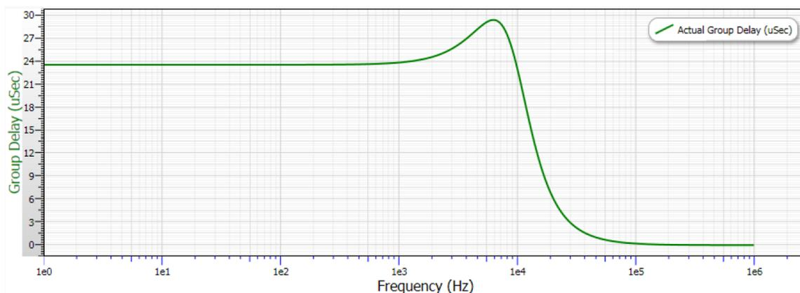
Figure 26. TIDA-01519 Antialiasing Filter Group Delay Plot
