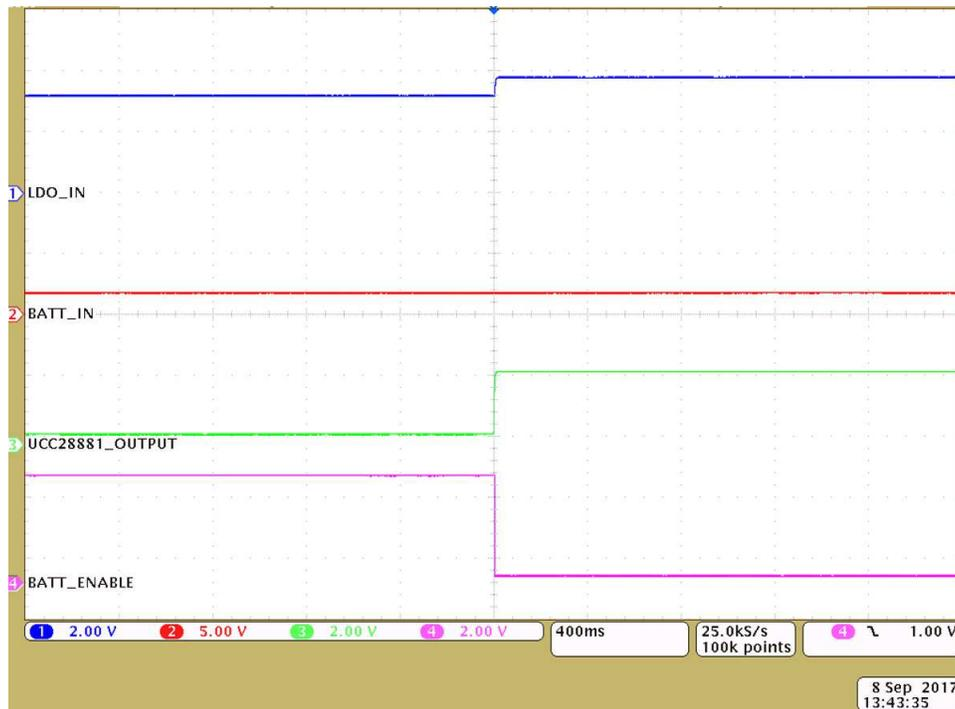
Figure 57. Test Results of Power ORing
