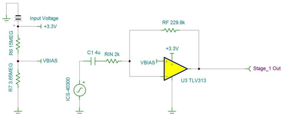
Figure 21. Active Filter and Gain Stage TINA-TI Simulation Schematic
