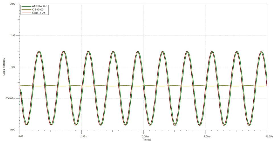
Figure 28. TINA-TI Simulation Output of TIDA-01519 Signal Chain
