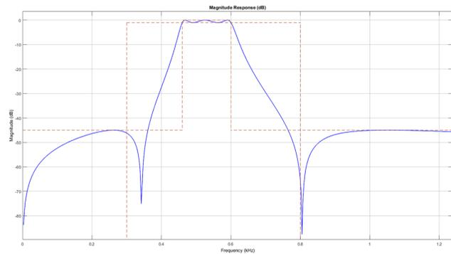
Figure 36. Magnitude Response of 520-Hz Digital Band-Pass Filter
