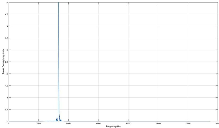
**Figure 37. Power Spectral Density Plot of 3-kHz Alarm at 2-ft Proximity**
