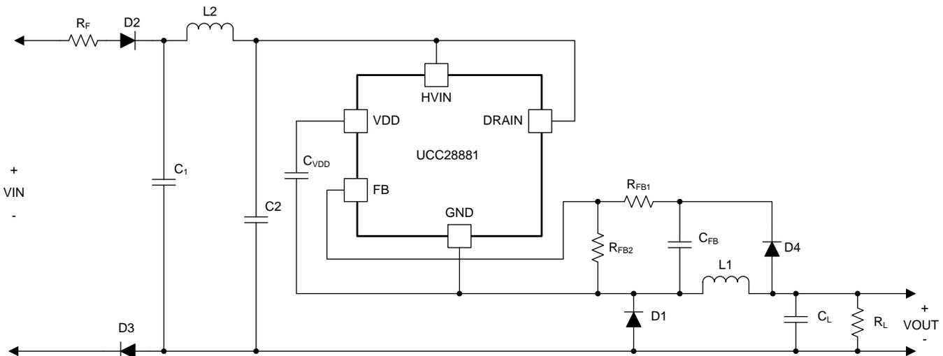
Figure 8. 120-V AC to DC Conversion Circuit, 3.9-V and 100-mA Output
