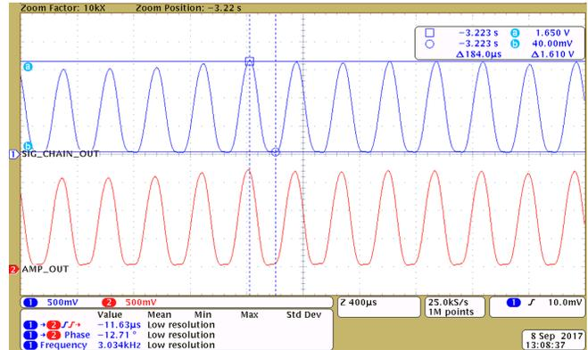
Figure 53. Delay, Phase, and Frequency Data Acquisition at 10-ft Proximity
