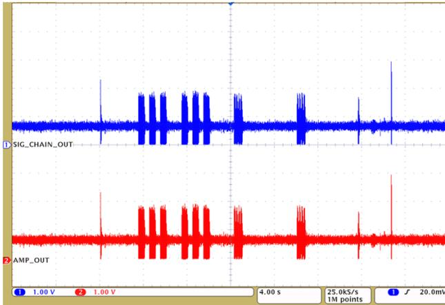
Figure 52. Signal Chain Response at 10-ft Proximity
