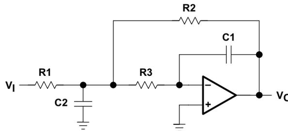
**Figure 23. Second-Order Unity Gain Sallen-Key Low-Pass Filter Topology**
