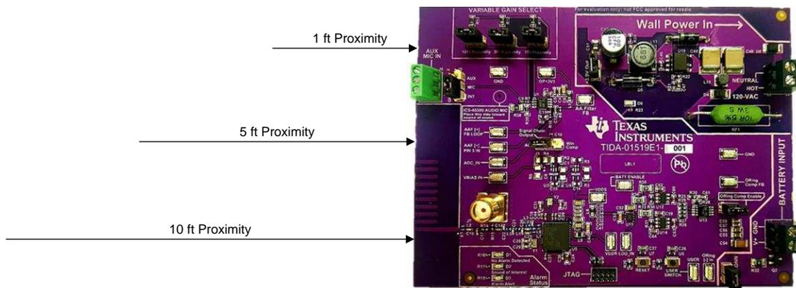
Figure 45. Test Setup of Audio Response Alarm
