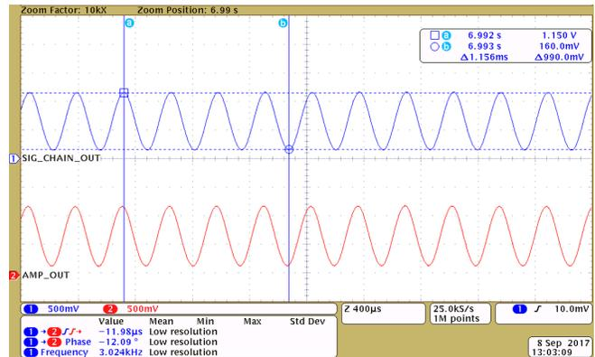
Figure 49. Delay, Phase, and Frequency Data Acquisition at 1-ft Proximity
