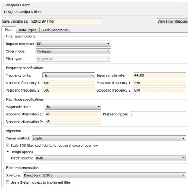
Figure 35. Parameter Definition of 520-Hz Digital Band-Pass Filter
