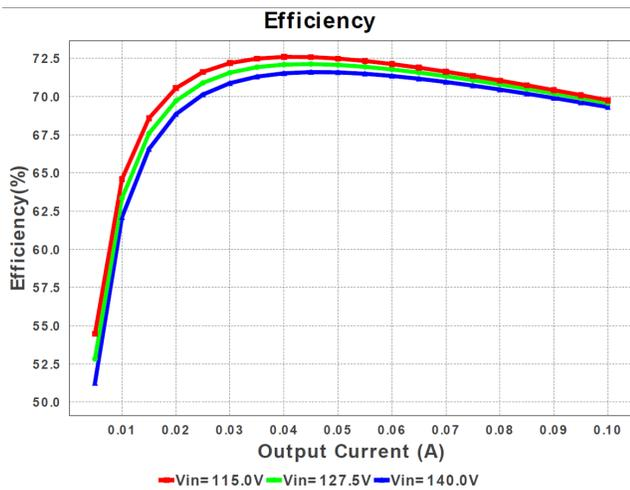
Figure 10. TIDA-01519 Efficiency Plot
