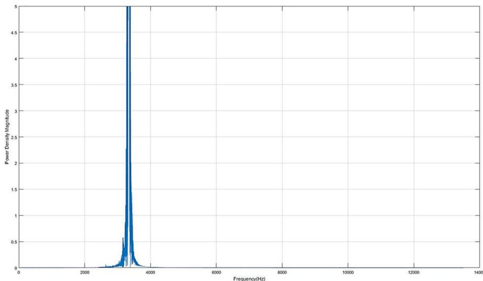
**Figure 38. Power Spectral Density Plot of 3-kHz Alarm at 10-ft Proximity**
