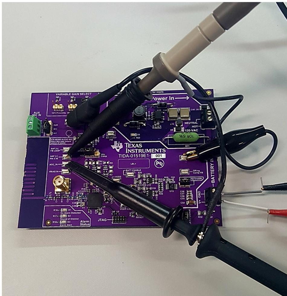
Figure 46. Setup of Audio Response Probe
