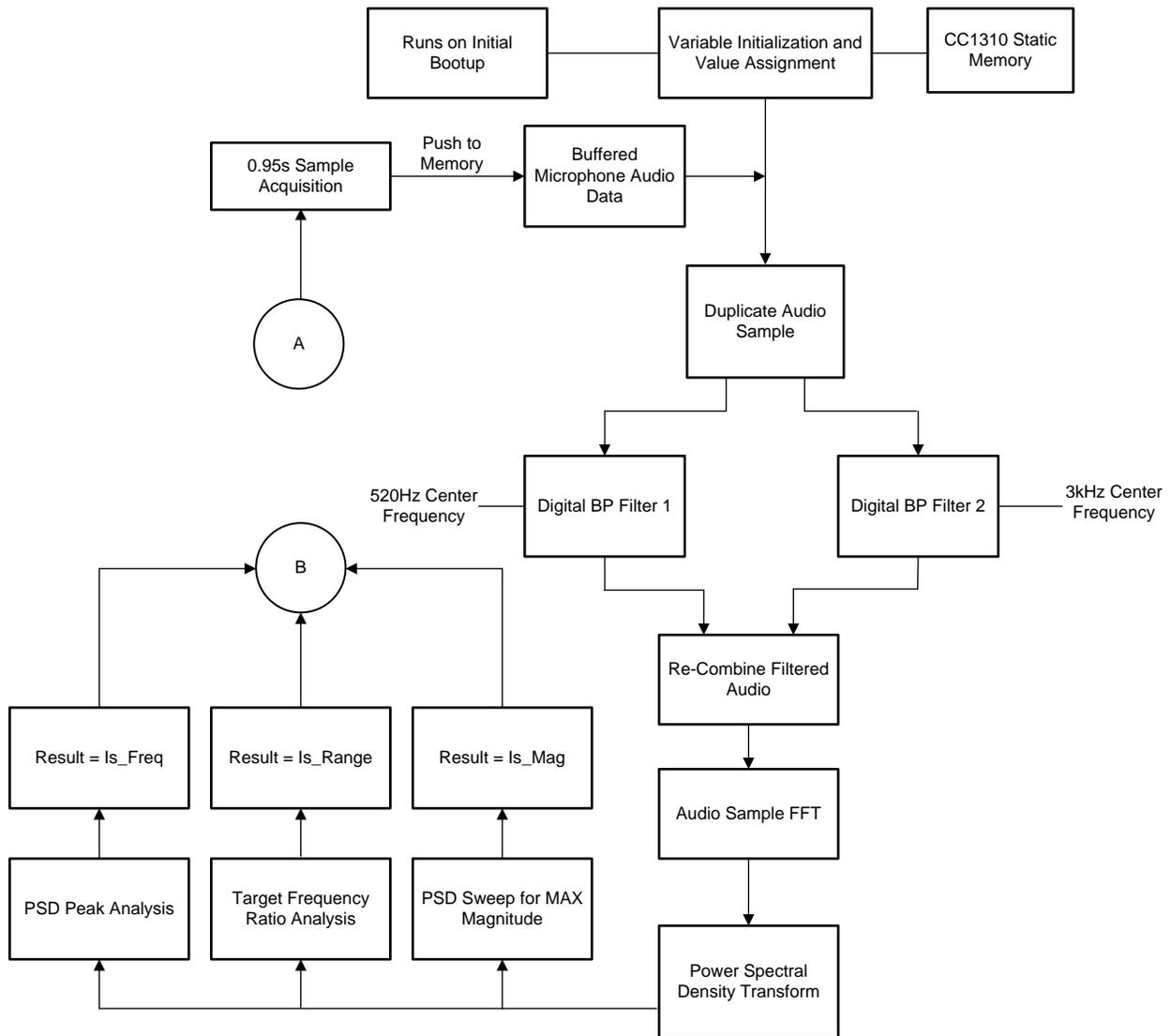
Figure 39. TIDA-01519 Audio Processing Flow Chart
