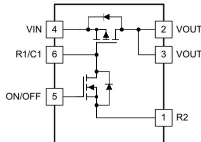
**Figure 6. TPS27081A Functional Block Diagram**
