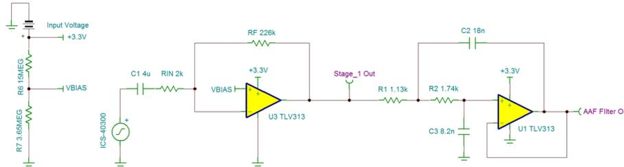
Figure 27. TIDA-01519 Signal Chain Simulation Schematic
