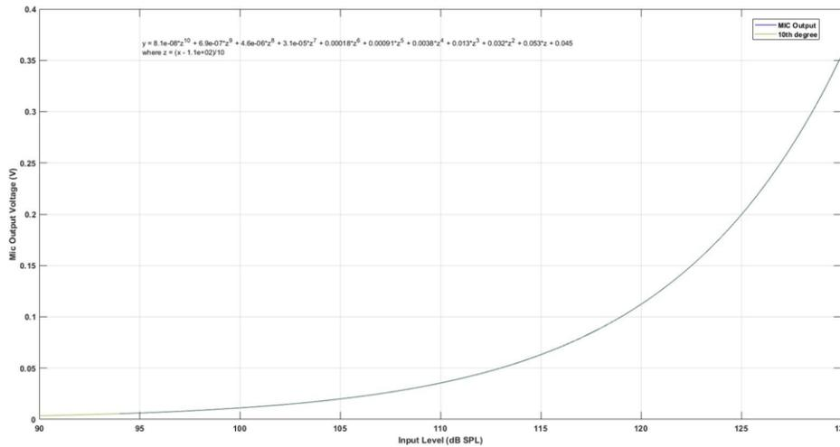
Figure 18. Microphone Voltage Output Using 10th Degree Poly-Fit Prediction Curve
