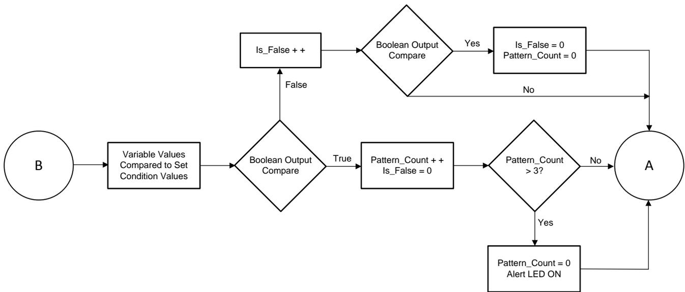
**Figure 40. TIDA-01519 Alarm Detection Algorithm Software Flow Chart**
