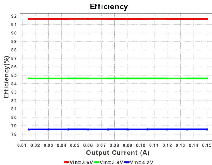
Figure 16. TPS780330220 Efficiency Curve Plot
