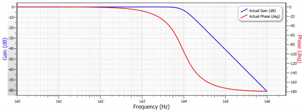
Figure 25. TIDA-01519 Antialiasing Filter Frequency Response Plot
