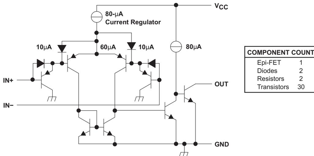
Figure 7. LM2903DGKR Functional Block Diagram
