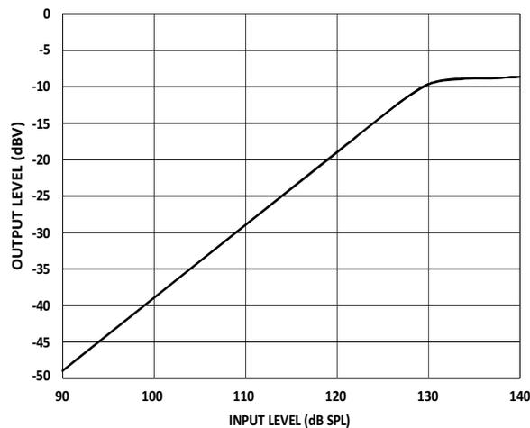
**Figure 17. ICS-40300 dBV Output Curve**
