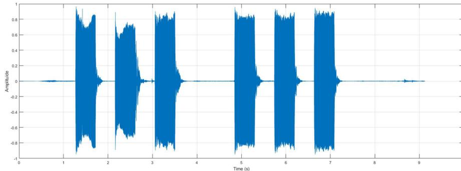
Figure 31. 3-kHz Fire Alarm Captured Audio Sample
