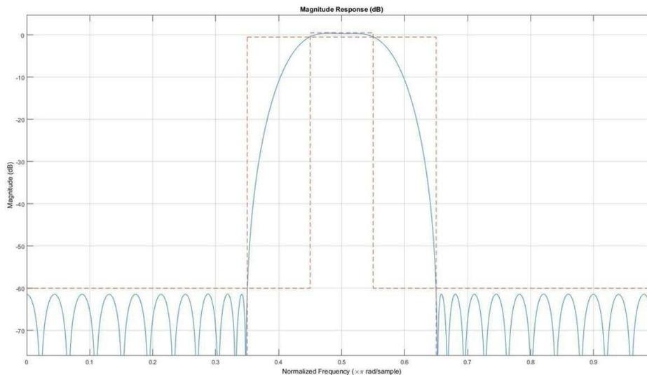
Figure 34. Magnitude Response of 3-kHz Digital Band-Pass Filter
