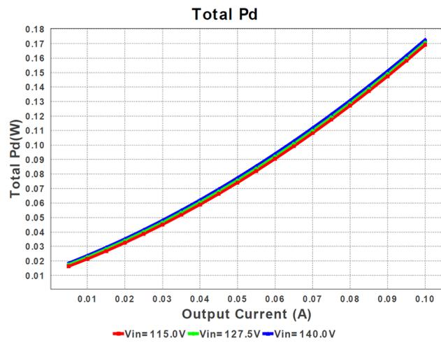
Figure 11. TIDA-01519 Total Power Dissipation Plot
