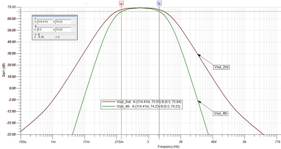
Figure 9. Frequency Response Dual vs Quad Stages (Linear Scale)
