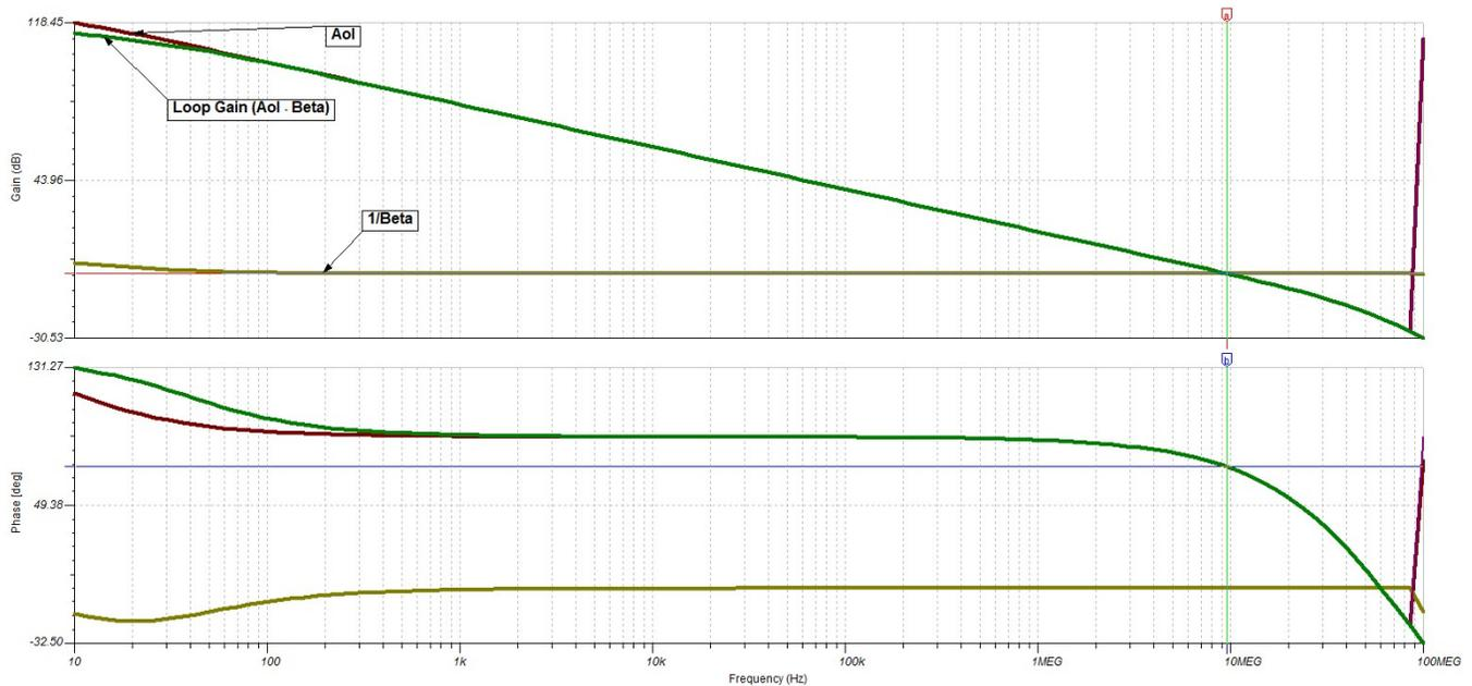
Stage-4 is exactly the same as stage-3, so the phase margin also remains the same. [Figure 16](#), [Figure 18](#), and [Figure 20](#) show the small signal stability frequency response of the circuit. As [Figure 17](#), [Figure 19](#), and [Figure 21](#) show, all amplifier stages (Stage-1, Stage-2, Stage-3, and Stage-4) of the signal conditioning circuit are stable with a phase margin of greater than 72°, respectively.
