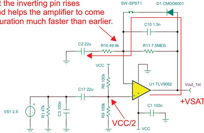
**Figure 15. Power-on Settling Time Simulation With Diode**
