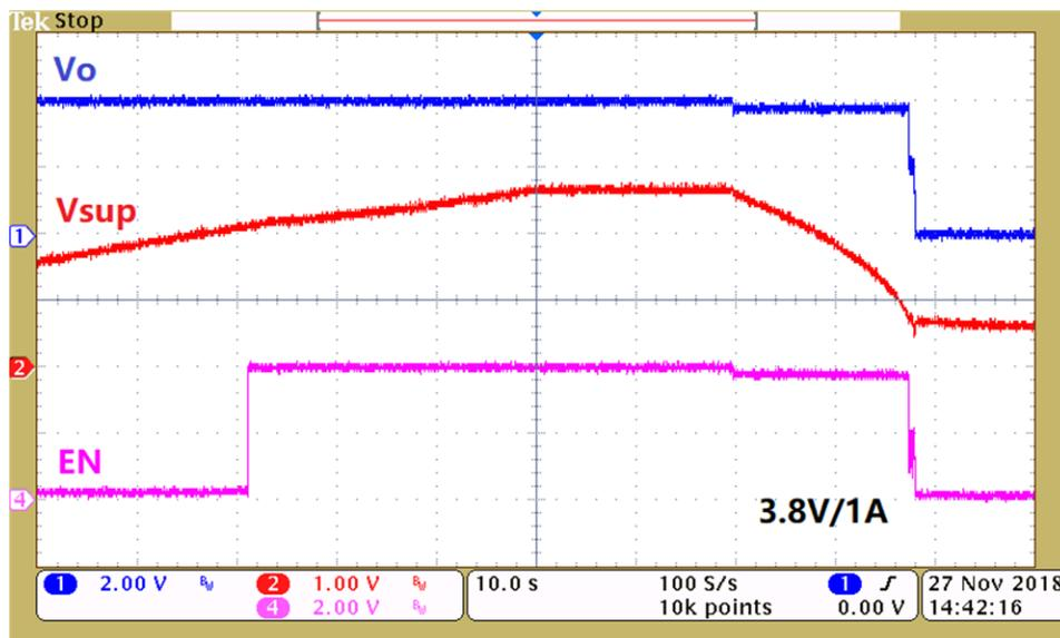
Figure 6. Working Sequence at  $V_o = 3.8\text{ V}$ ,  $I_o=1\text{ A}$
