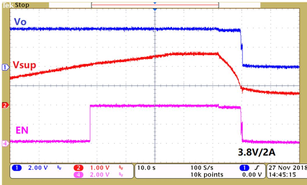
Figure 7. Working Sequence at  $V_o = 3.8\text{ V}$ ,  $I_o = 2\text{ A}$
