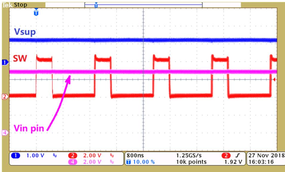
Figure 9. SW and VIN Pin Waveform When  $V_{sup} = 1.2\text{ V}$
