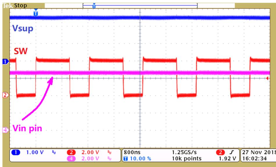
Figure 8. SW and VIN Pin Waveform When  $V_{sup} = 2.5\text{ V}$
