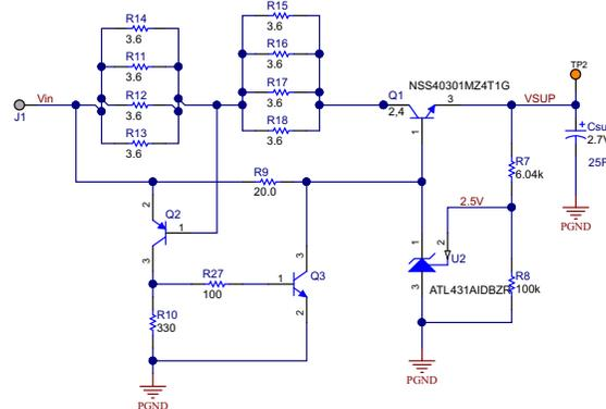
Figure 2. Super-Capacitor Charge Circuit
