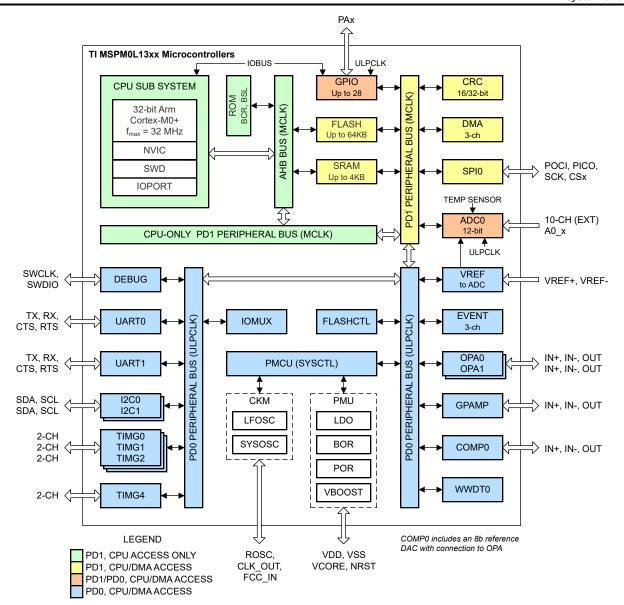
Figure 2-3. MSPM0L130x Functional Block Diagram
