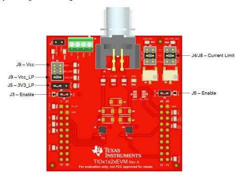
Figure 3-1. TIOx1x2xEVM Jumper Settings
