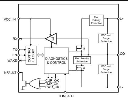
Figure 2-2. TIOL112 Block Diagram
