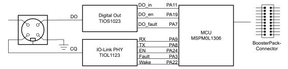
Figure 2-1. TIDA-010263 Block Diagram
