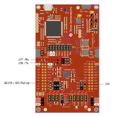
Figure 3-3. MSPM0L1306 LaunchPad™ Development Kit Jumper Settings
