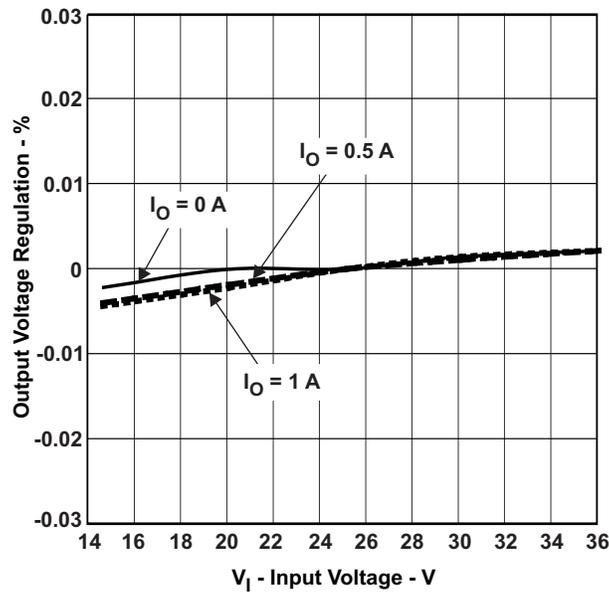
Figure 5. TPS5410 12 V Output Line Regulation
