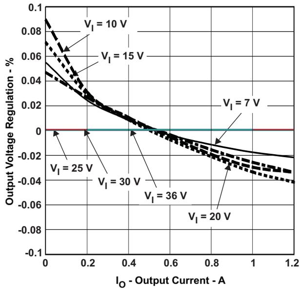
Figure 4. TPS5410 5 V Output Load Regulation
