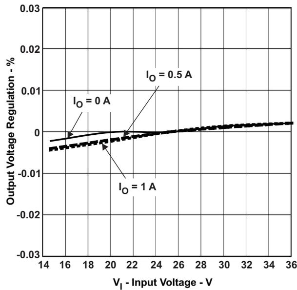
Figure 6. TPS5410 5 V Output Line Regulation
