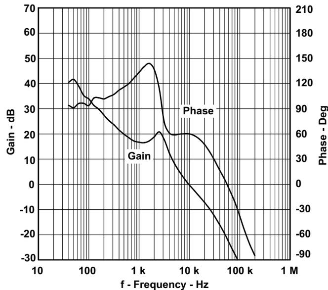
Figure 9. TPS5410 12 V Output Loop Response
